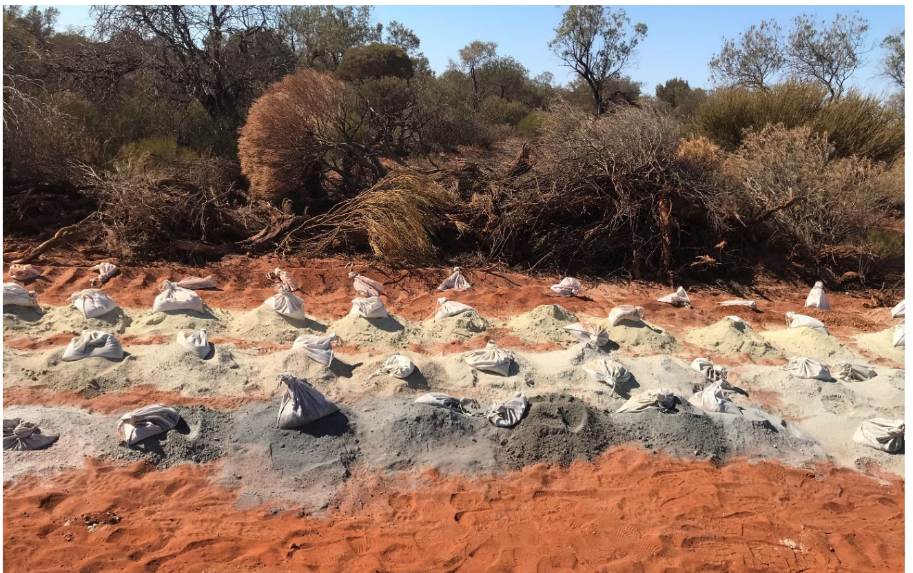
Photo 2: Drill hole CORC027 samples showing part of gold mineralised interval 92 to 100m
