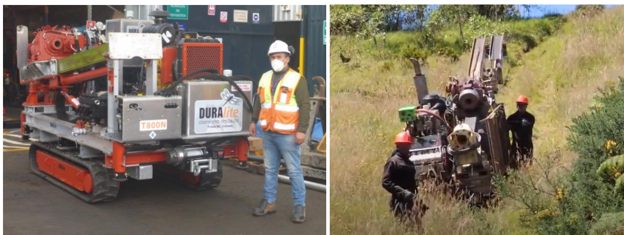
Figure 2 ABOVE LEFT: The intended drill rig for Riqueza. ABOVE RIGHT: The drill rig model in the field (not Riqueza). The need for elaborate access tracks is negated because the rig is light weight and track mounted. It still has the capacity to drill over 1,000m depth.
