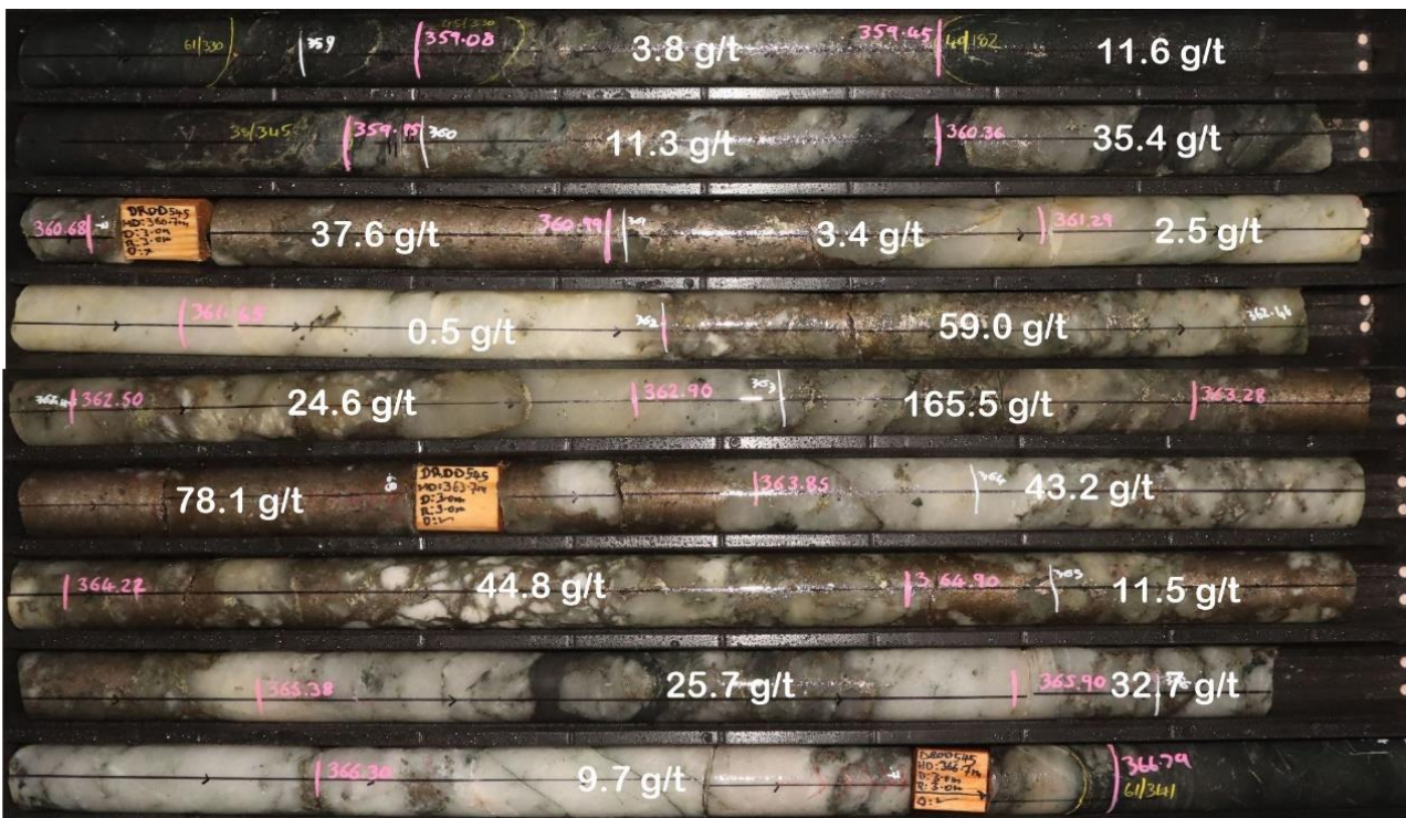
Figure 3: DRDD545 Recent core from the Armand Lode, 40m step out hole north of previous drilling. Milky quartz veining with narrow zones of smokey grey quartz. There are roughly equal amounts of 25% semi massive pyrrhotite and trace chalcopyrite fracture fill. 140+ flecks of visible gold logged throughout the interval. Interval assayed 8.3m @ 32.1 g/t gold from 358.5m
