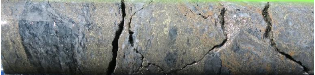
OFDD003: sheared quartz vein with semi-massive pyrite-sphalerite-galena (277.4 - 277.6m)
