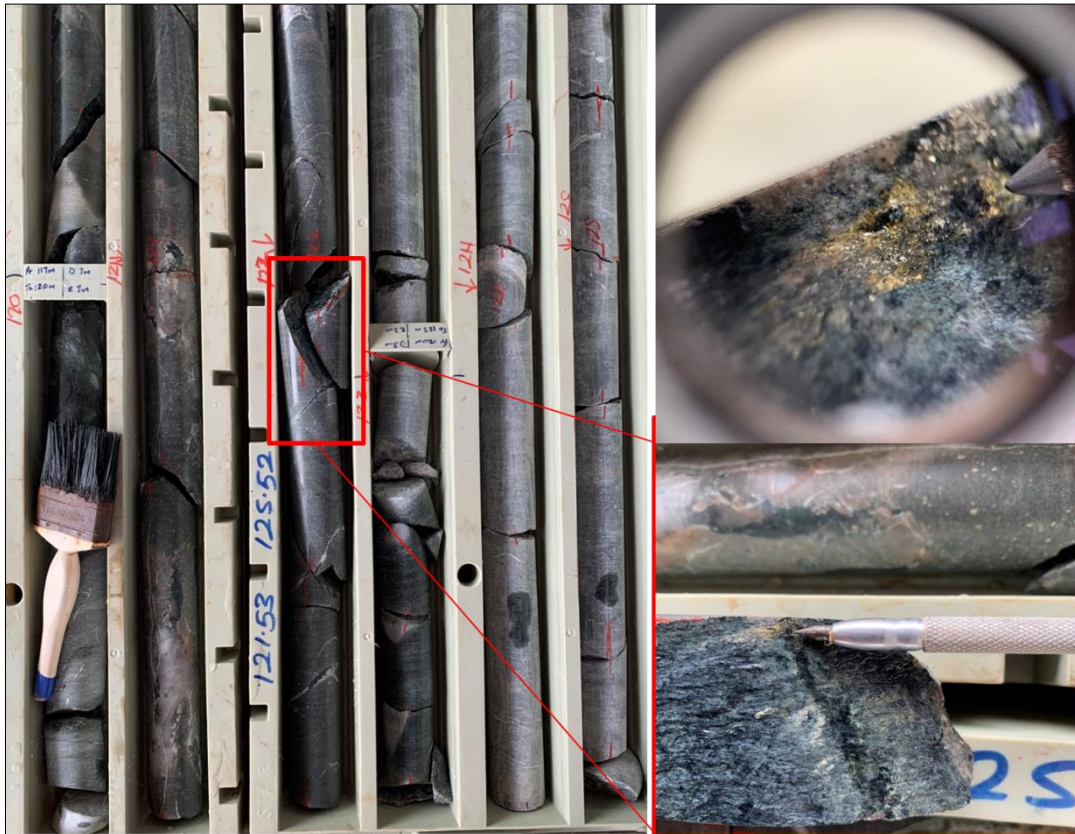
Figure 6: SDD196 from 119.5m to 125.5m with strong silica+albite alteration, euhedral coarse pyrite and visible gold at 121.95m.
