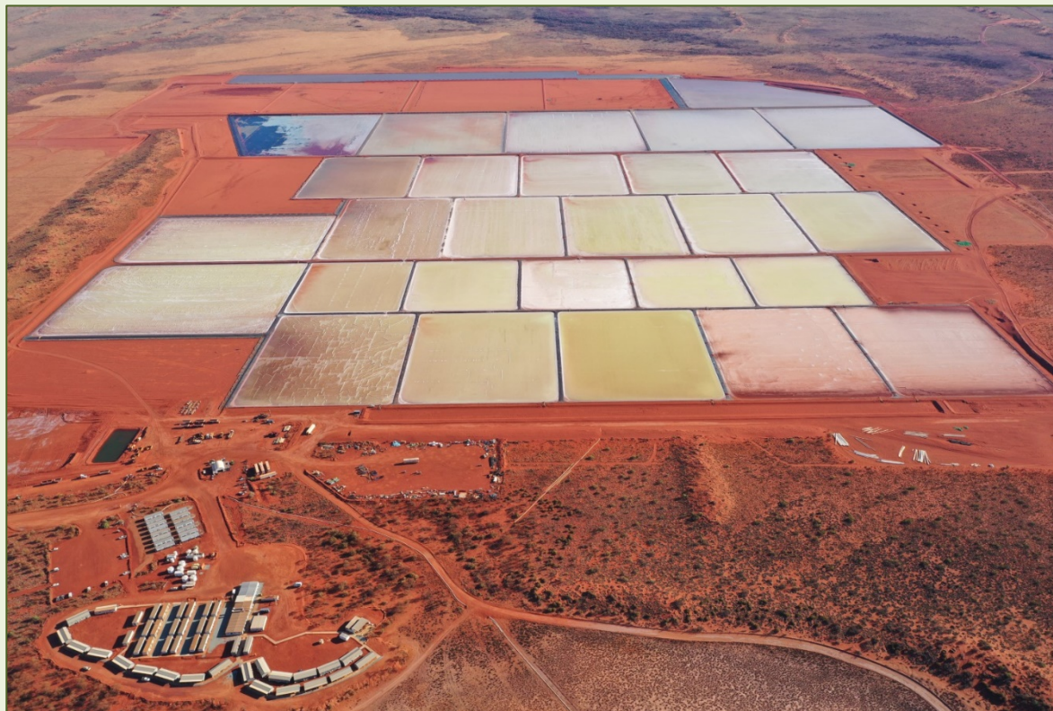
Crystalliser Ponds Progressively Being Built, Lined and Brine Filled
