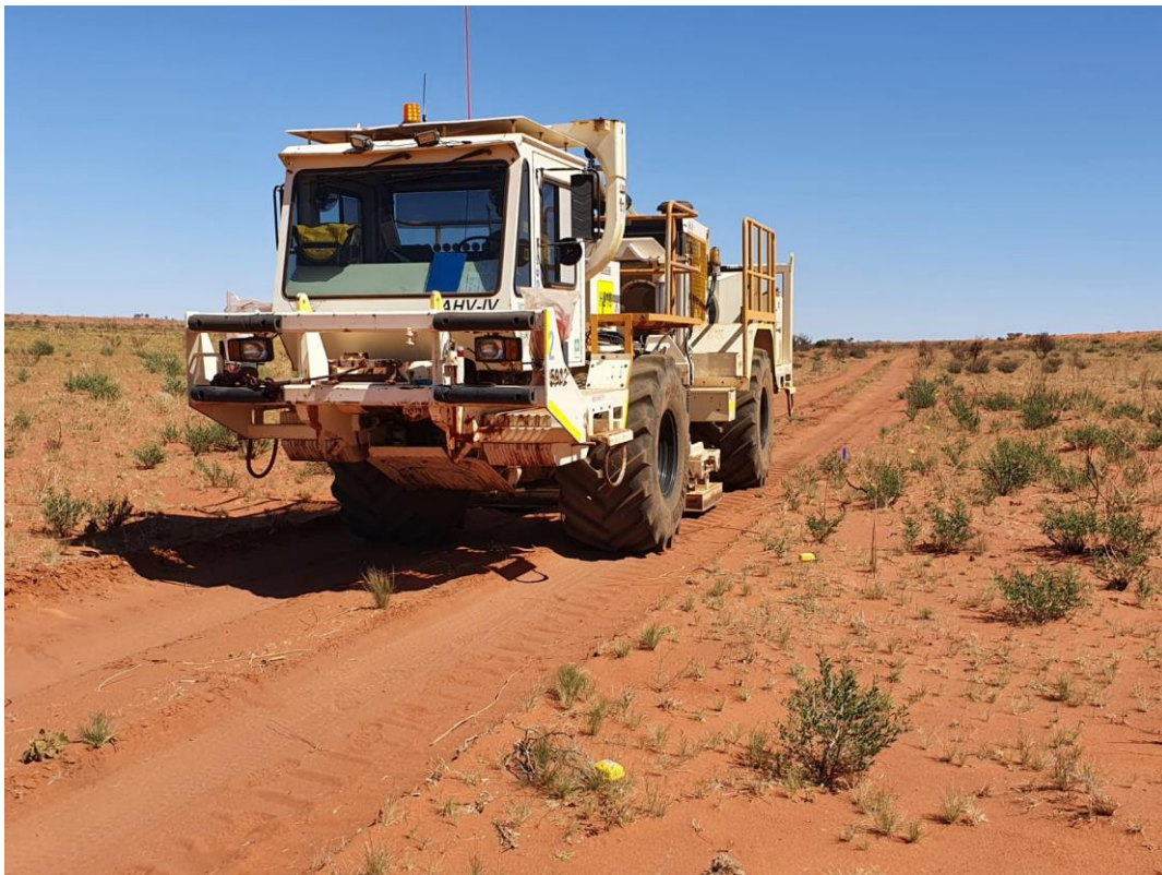
Figure 2 Hiseis Inova AHV-1V 62,000lb seismic vibrator truck with Inova Quantum receiver nodes layed every 5m along the track
