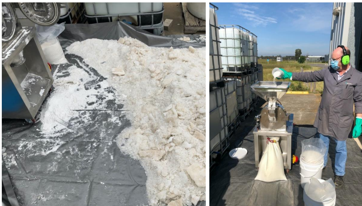
Figure 2: (a) Crushing of potassium enriched mixed salts from KLPP, (b) Fine milling of mixed salts.
