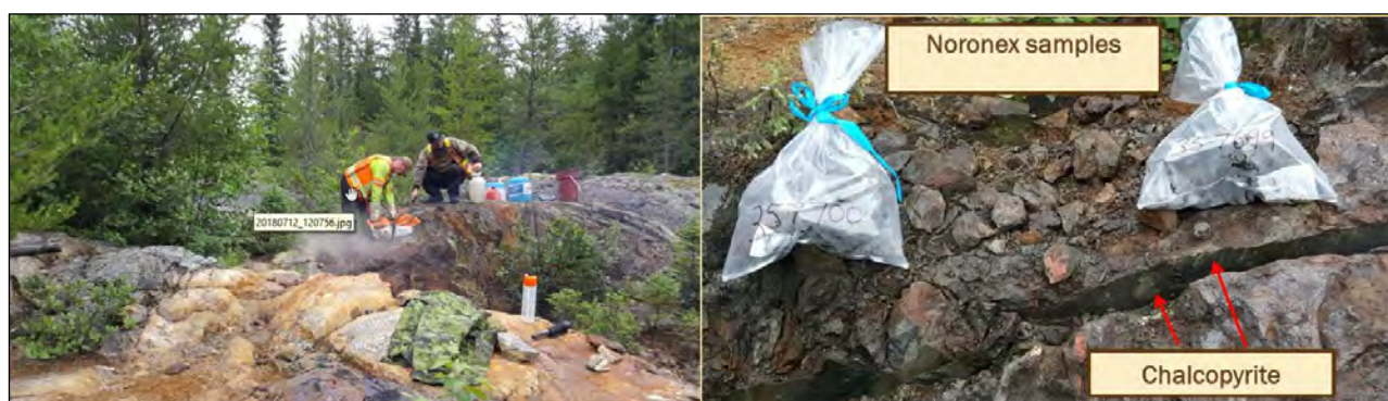
Figure 26: Photographs of channel sampling of massive sulphide mineralisation in Perry trench by Noronex Source: Noronex Ltd
