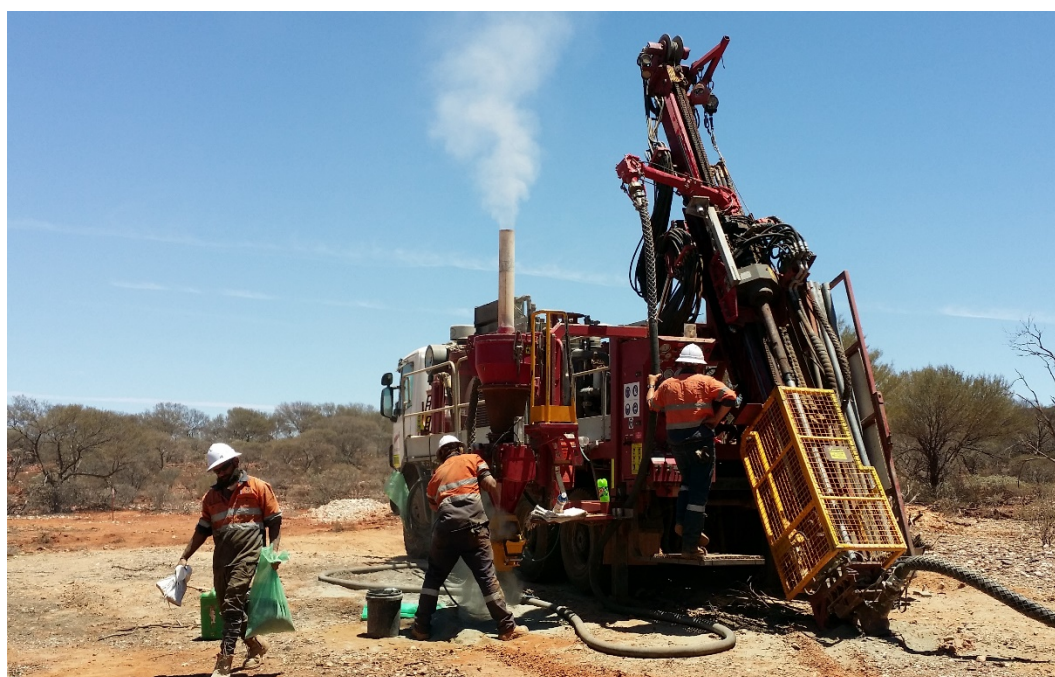
Photo 1: RC drill rig at Reedy South
