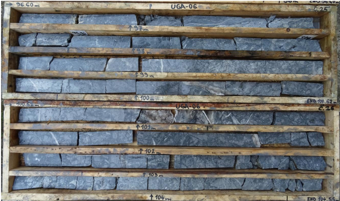
Figure 10: UGA-06 drill core; interval from 96.6m to 104.55m (down-hole) showing quartz filled vein/stockwork/breccia structures, variably rich in fine to very fine grained sulphides (mainly pyrite/marcasite) and hosted within strongly argillic altered andesite host rock. Traces of visible gold identified between 98-100m
