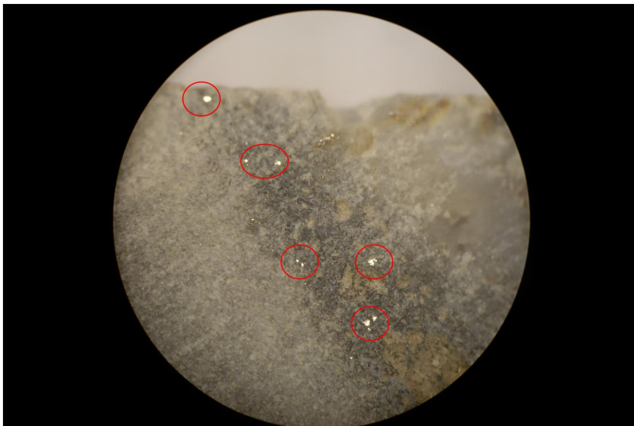
Figure 5: Stereoscope image of the visible gold at 62.4m associated with pyrite (x20 magnification: field of view is ~10mm) in UGA-06
