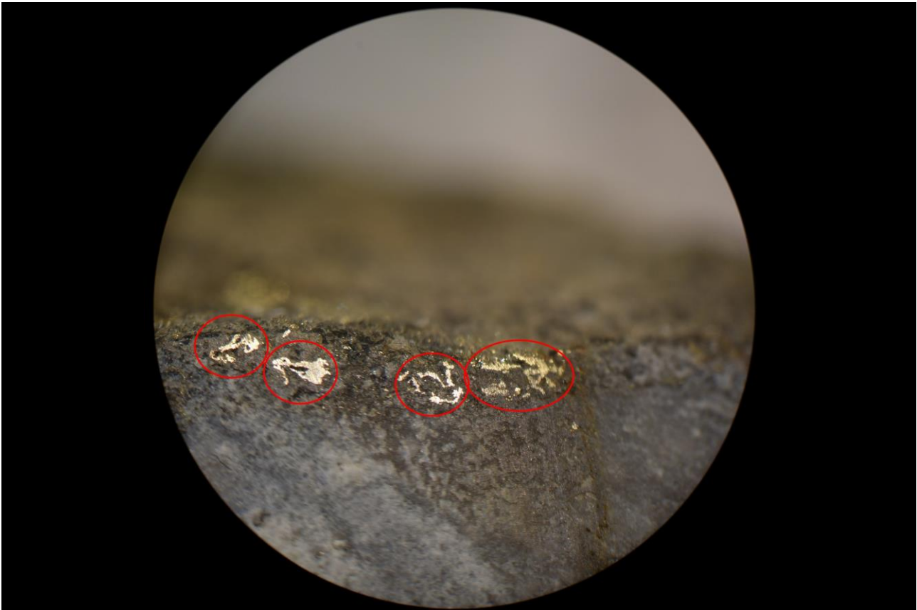
Figure 2: Stereoscope image of the visible gold at 40.5m associated with pyrite (x40 magnification: field of view is ~5mm) in UGA-06
