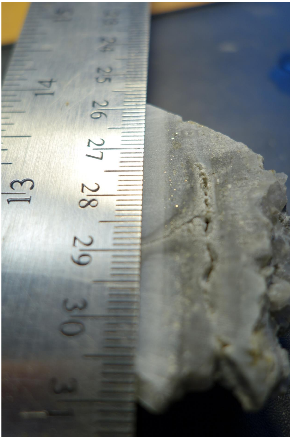
Figure 4: Chalcidonic vein with traces of visible gold and pyrite at approximately 62.4m in UGA-06 (close up of visible gold shown in Figure 5)
