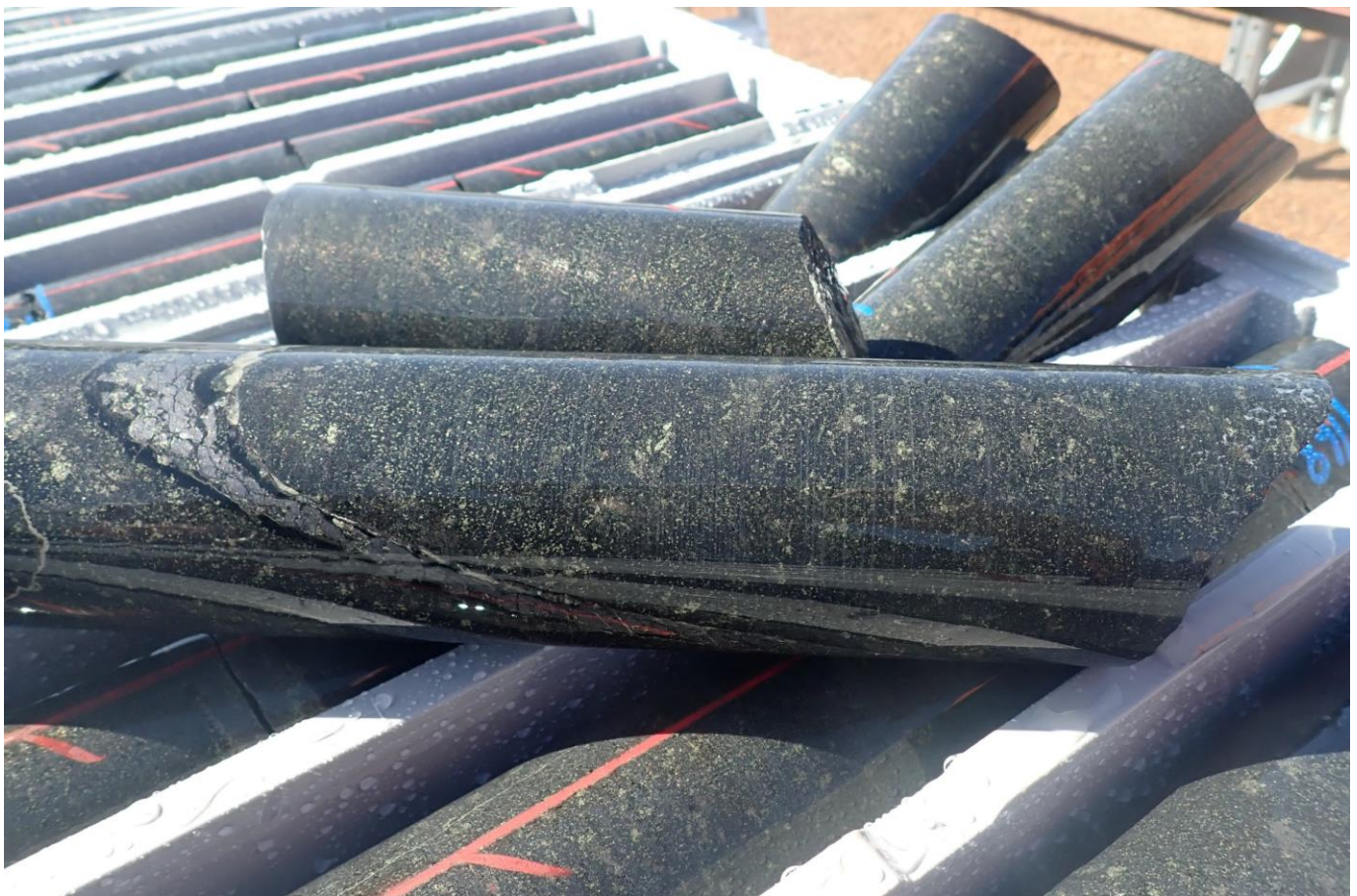
Figure 4. JD019 drill core specimens – heavily disseminated chalcopyrite +/- pyrrhotite sulphides from 141m down-hole.
