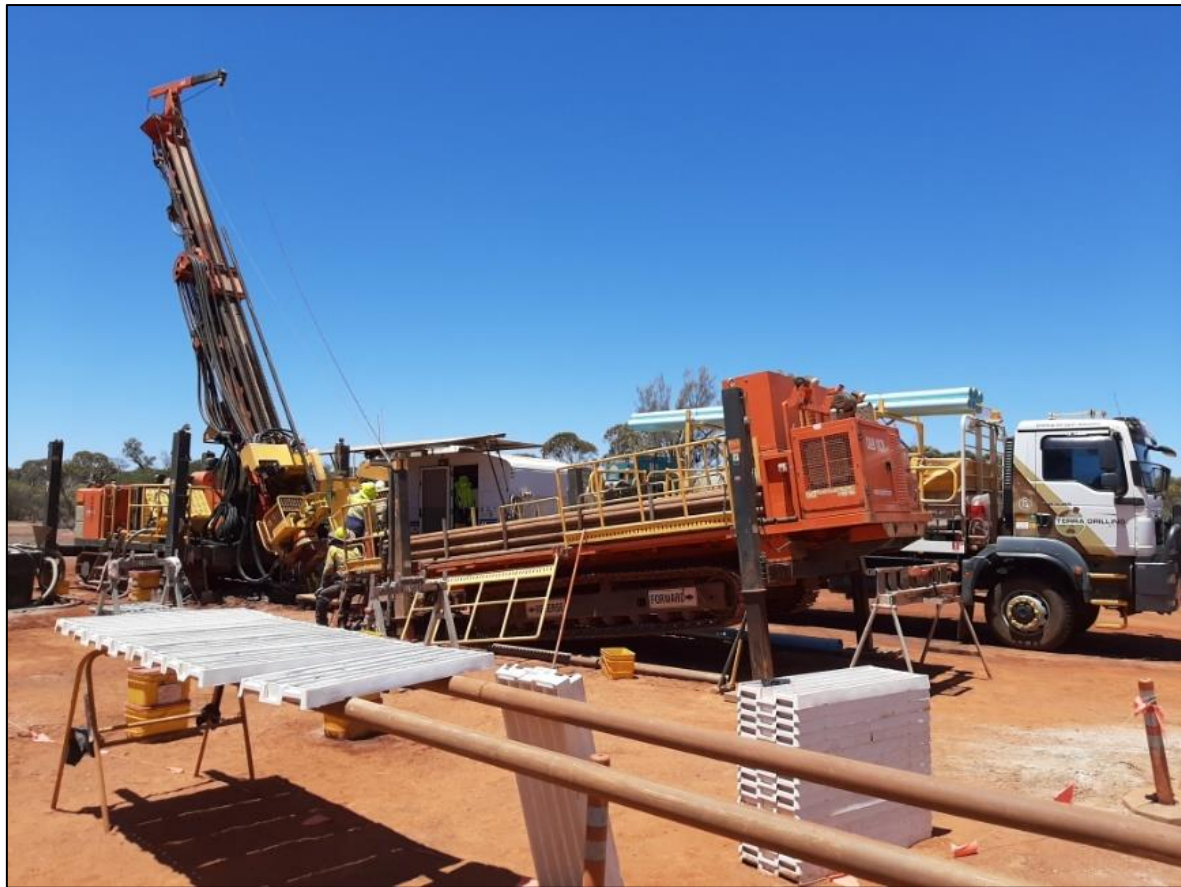
Figure 3 – Drilling the first diamond hole (GDDD001) at the Gordons Dam gold prospect.
