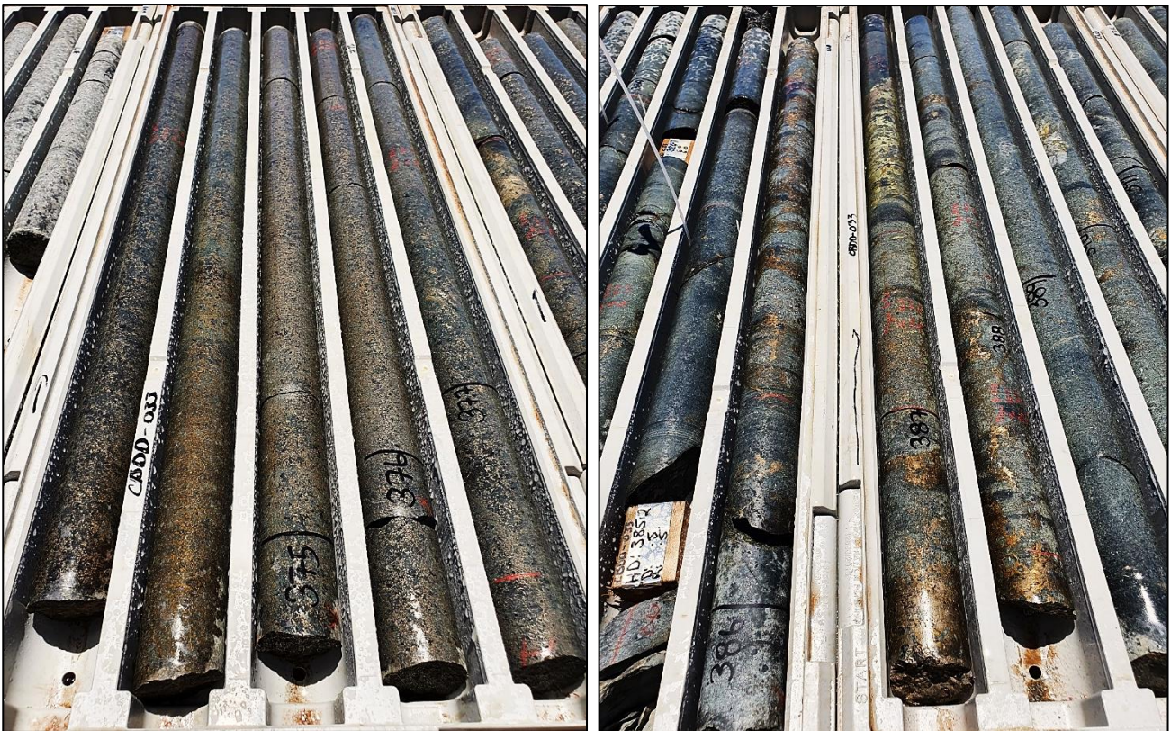
Figure 2. Ni-Cu bearing matrix-massive sulphide zone in upper zone (left image) and breccia sulphides in lower sulphide zone (right image) within diamond drill hole CBDD033 at the T5 Ni-Cu discovery (373.2-377.8m & 385.0-391.3m shown).
