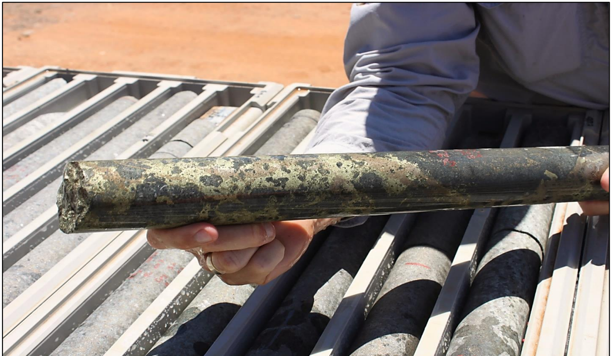
Figure 1. Copper rich breccia sulphides (chalcopyrite+pyrrhotite) towards the base of a 25.7m wide zone of Ni-Cu mineralisation within drill hole CBDD033 at the T5 Prospect, Carr Boyd Rocks Project (387.2m-387.8m shown).
