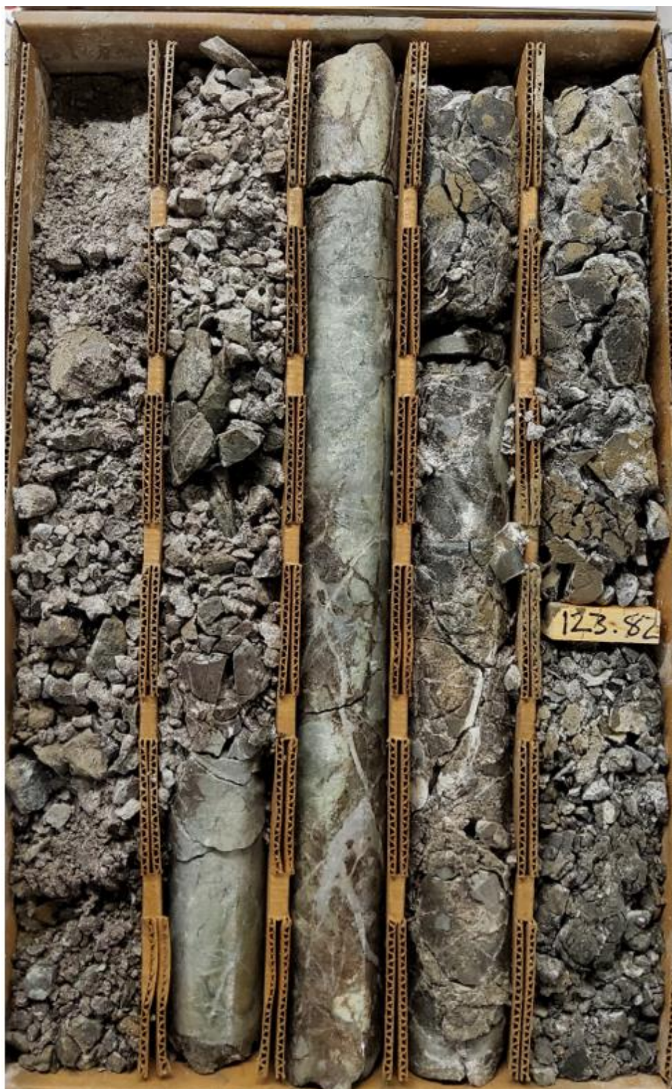
Figure 9: Hole DD20M-003 (Site D), downhole depth from 121.6m to 124.0m. Block of Pyroxene Skarn interdigitated with strongly altered Diorite. Diorite has potassic alteration overprinted by phyllic. Both lithologies are Argillically altered. Quartz sulfide veins contain abundant pyrite and traces of chalcopyrite. Magnetic susceptibility measurements of this interval showed values less than 7 units. Assay results for DD20M-003 are pending.
