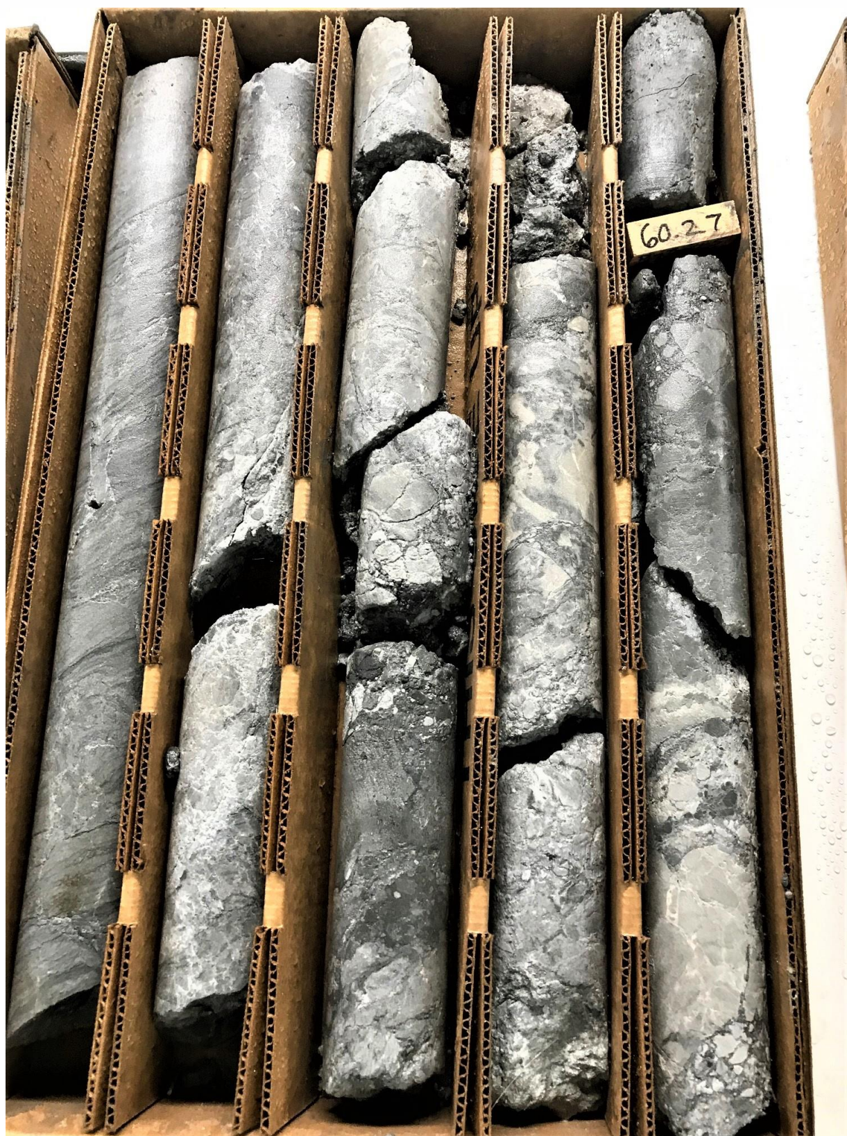
Figure 6: Hole DD20M-002 (Site H redrill), downhole depth from 57.8m to 60.3m. Tatow Limestone (Cpt) Moderate to local Strong Carbon-Clay-Pyrite Breccia throughout. Deformation is interpreted to be related to regional-scale compressional faulting and hydrothermal dissolution. Refer Table 1 for initial assay results, remaining assay results from DD20M-002 are pending.
