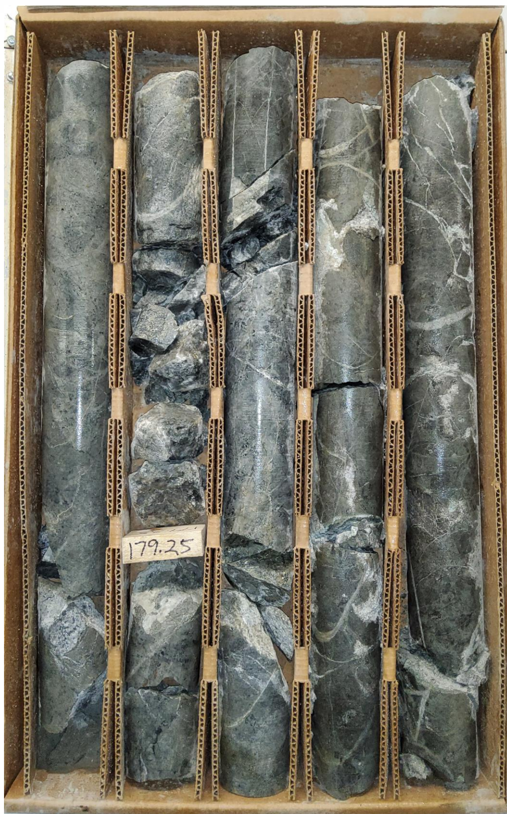
Figure 7: Hole DD20M-003 (Site D), downhole depth from 178.5m to 180.9m. Diorite displaying early brownish-green, magnetite-bearing, potassic alteration overprinted by lighter-colored phyllic alteration that is related to abundant quartz-sulfide veins. Pyrite >>Molybdenite>>Chalcopyrite. Magnetic susceptibility measurements of this interval showed values of about 35 units. Assay results for DD20M-003 are pending.
