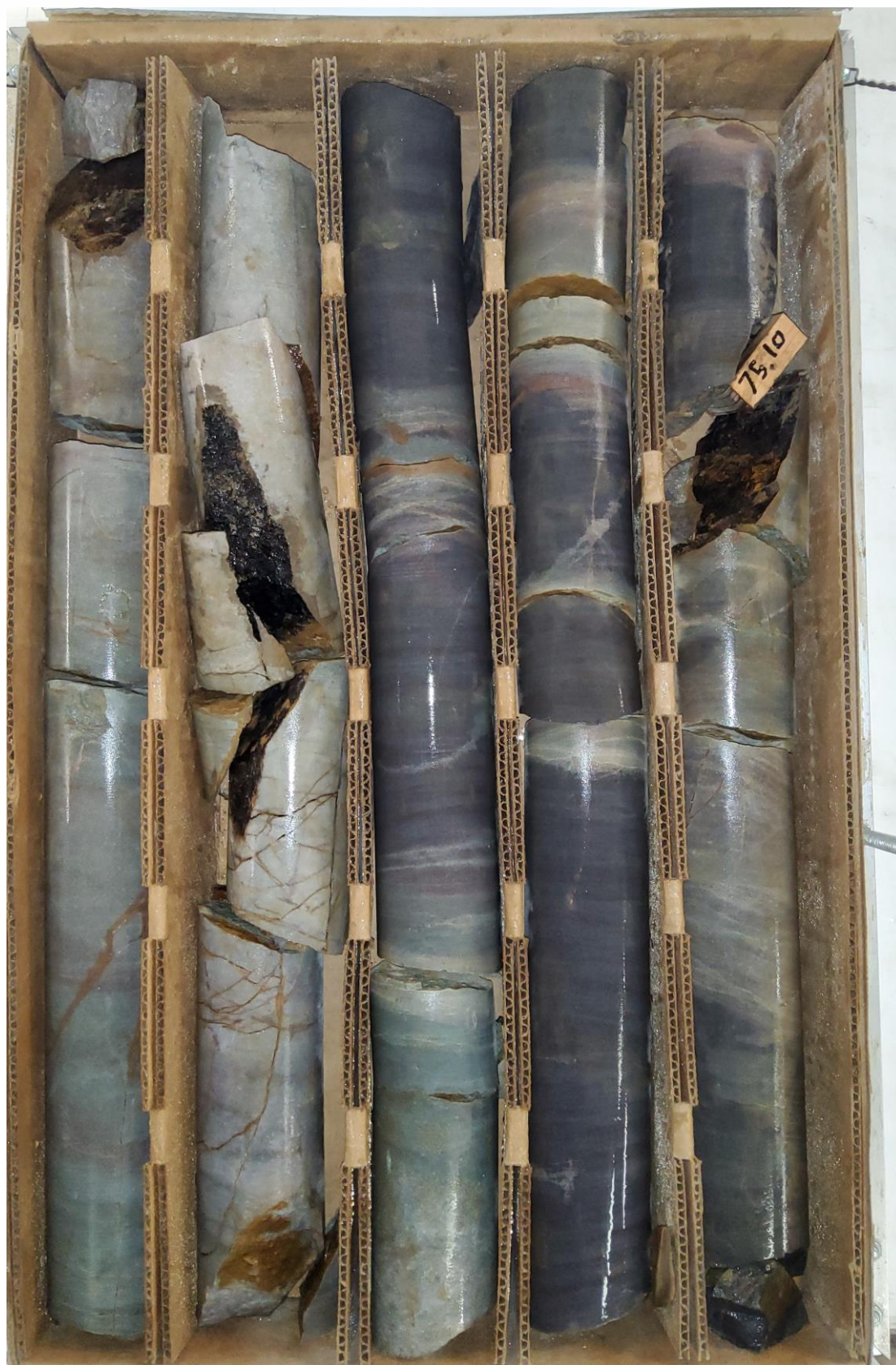
Figure 10: Hole DD20M-005(Site I), downhole depth from 72.7m to 75.3m. Altered and iron-oxide mineralized quartzite. Bleached area cross-cutting hematite-chlorite cemented quartzite represents fracture-controlled quartz-sericite-pyrite (phyllic) alteration that has been weathered to Goethite by surface waters. Example of postulated “Marigold-style” mineralization. Assay results for DD20M-005 are pending.
