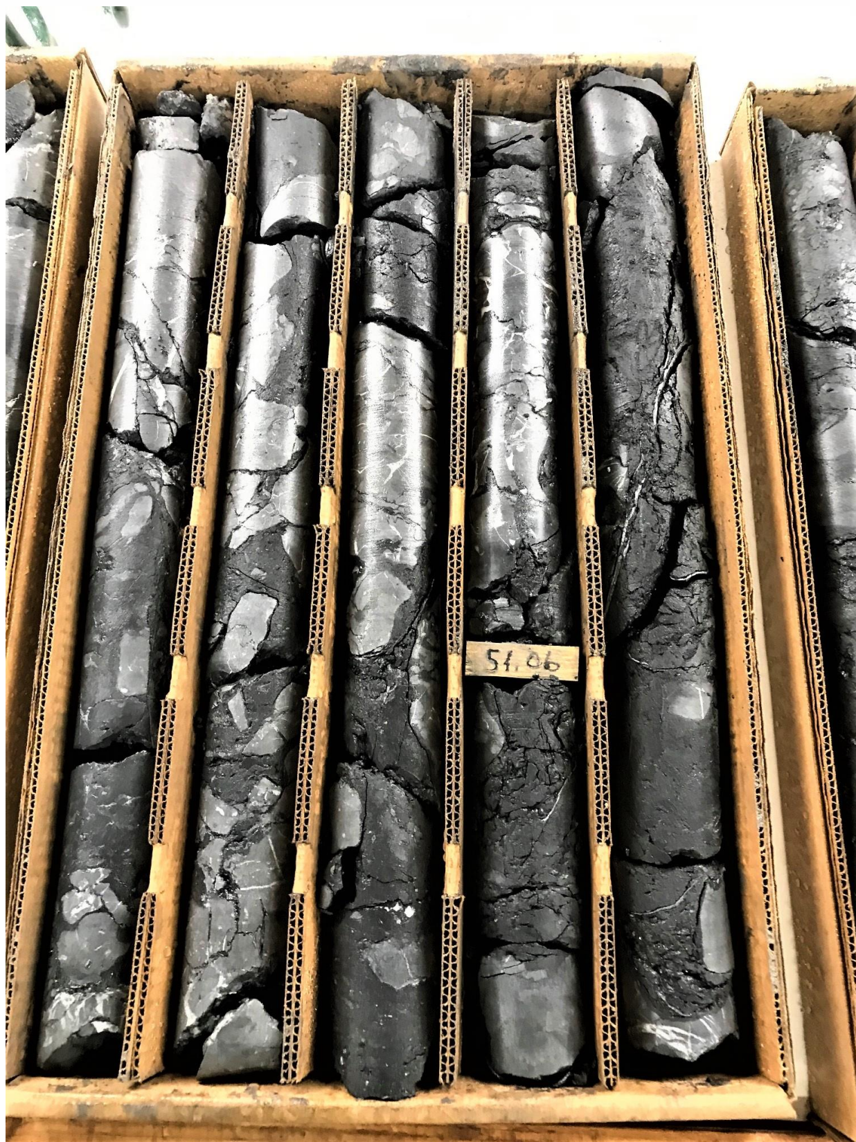
Figure 5: Hole DD20M-002 (Site H redrill), downhole depth from 49.2m to 52.1m. Tatow Limestone (Cpt) Moderate to local Strong Carbon-Clay-Pyrite Dissolution Breccia throughout. Refer Table 1 for initial assay results, remaining assay results from DD20M-002 are pending.
