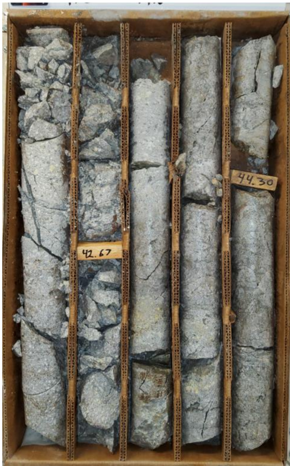
Figure 8: Hole DD20M-004 (Site C), downhole depth from 41.8m to 44.6m. Monzonite porphyry displaying strong phyllic alteration composed fine grained sericite-quartz-pyrite overprinted by argillic (sticky white clay) alteration. This core is competent due to strong quartz flooding and contains 10% fine-grained pyrite and trace amounts of exceptionally fine grained, dark grey sulfosalt mineral. Assay results for DD20M-004 are pending.
