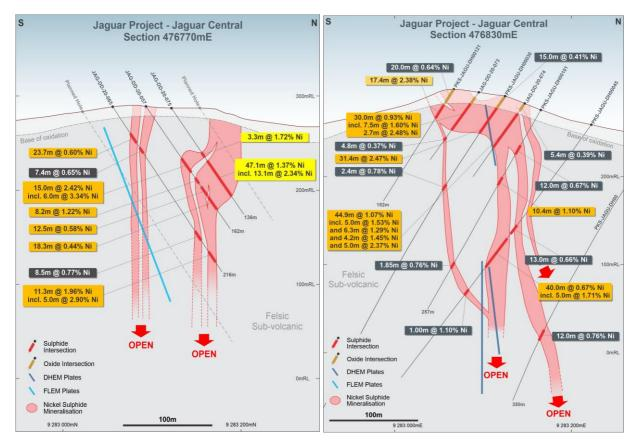
Figure 3 – The Jaguar Central Deposit: Cross-Sections 476980mE (left) and 477080mE (right) showing the drill intersections with DHEM conductor plates in dark blue and FLEM plates in light blue.
