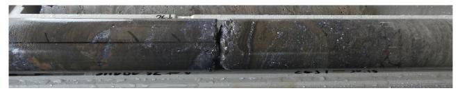
Figure 6: Example of stratiform galena mineralisation intersected in SHDD032 at approximately 27m down hole depth.
