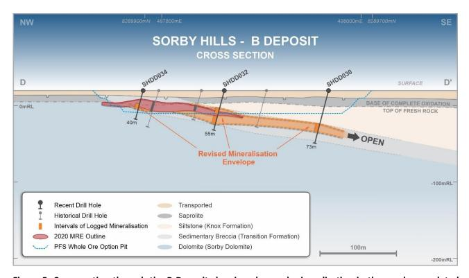
Figure 5: Cross section through the B Deposit showing observed mineralisation in the newly completed drill holes SHDD030, SDDSH032 and SHDD034 relative to the current Resource envelope and open pit design.
