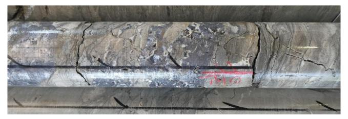
Figure 4: Example of stratiform galena mineralisation interval intersected in SHDD043 at approximately 68m down hole.
