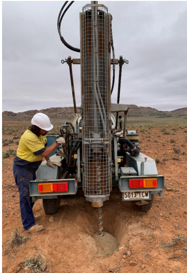
Figure 9: Auger Drilling of Hematite-Altered (Miox) Dolerite Within the Newly Discovered Outcropping Mineralised Breccia at Jenkins South.
