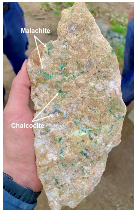
Figure 5: Sample WK0651: Chalcopyrite, Chalcocite and Malachite Found in Massive Calcite Boulders within the Newly Discovered Mineralised Breccia at Jenkins South. Sample Returned Anomalous Copper Results of 0.65% Cu.
