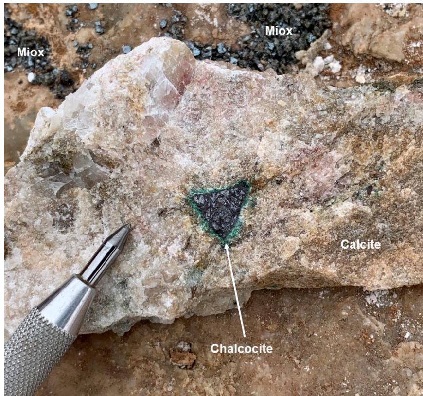
Figure 7: Chalcocite with Malachite Halo Found in Massive Calcite Boulders within the Newly Discovered Mineralised Breccia at Jenkins South. Note Miox in the background.
