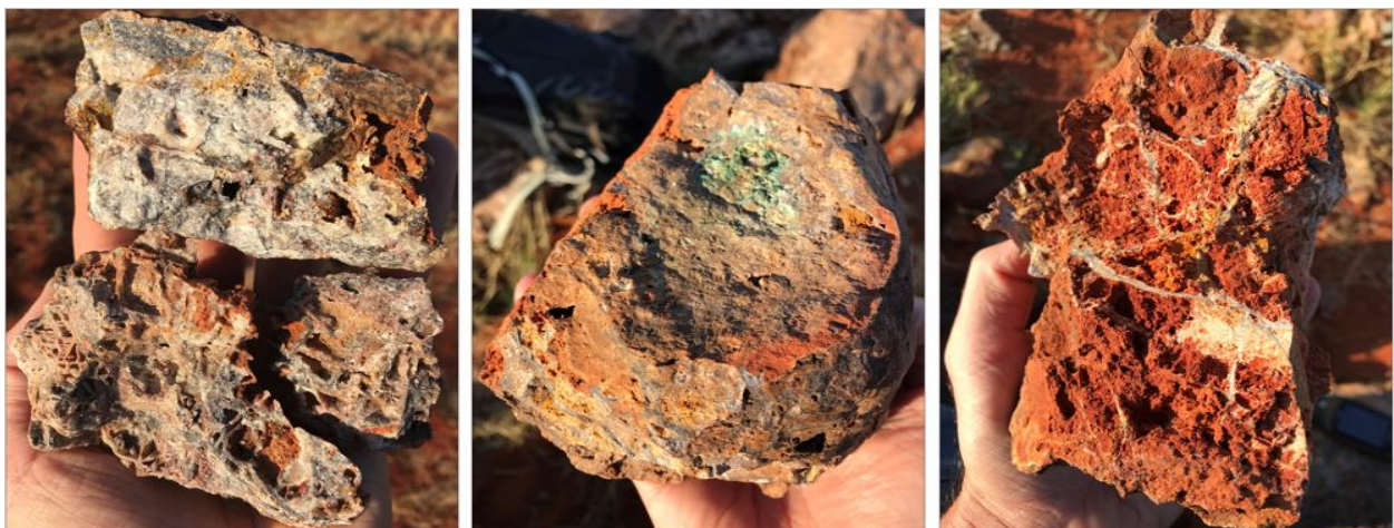
Figure 7: Examples of Sunset Boulevard Cu enrichment. ABOVE LEFT: Sample JE0046 quartz stockwork with limonite and oxide cemented fractures with 1,110ppm Cu; ABOVE MIDDLE: Sample JE0047 heavily quartz-hematite veined ex-granite with malachite and limonite with 5,250ppm Cu; ABOVE RIGHT: Sample JE0048 quartz-hematite stockwork ex-granite with 3,380ppm Cu (0.34% Cu).
