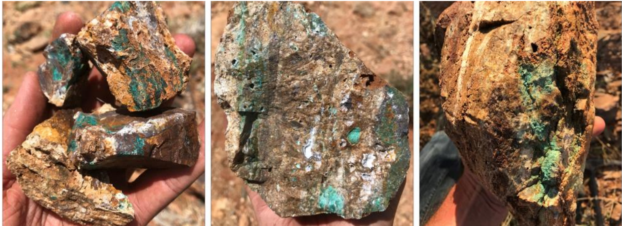
Figure 4: Examples of Ningaloo mineralisation. ABOVE LEFT: Sample JE0074 malachite-azurite with quartz and Fe-oxides with 3.92% Cu; ABOVE MIDDLE: Sample JE0075 malachite-azurite with quartz and Fe-oxides with 2.47% Cu + 2.71g/t Ag; ABOVE RIGHT: Sample JE0045 malachite-azurite with quartz with 10.3% Cu + 3.8g/t Ag.
