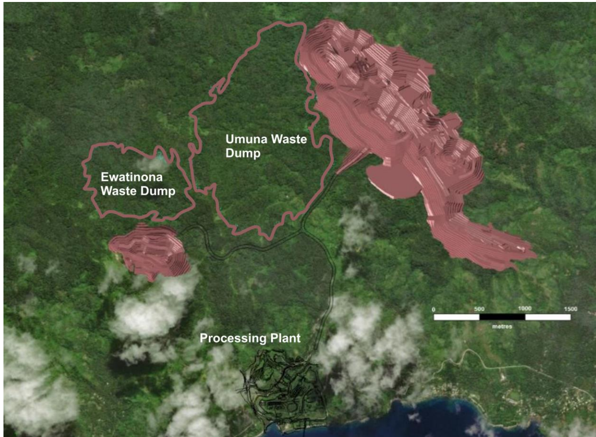
Figure 10: Waste Rock Dumps
