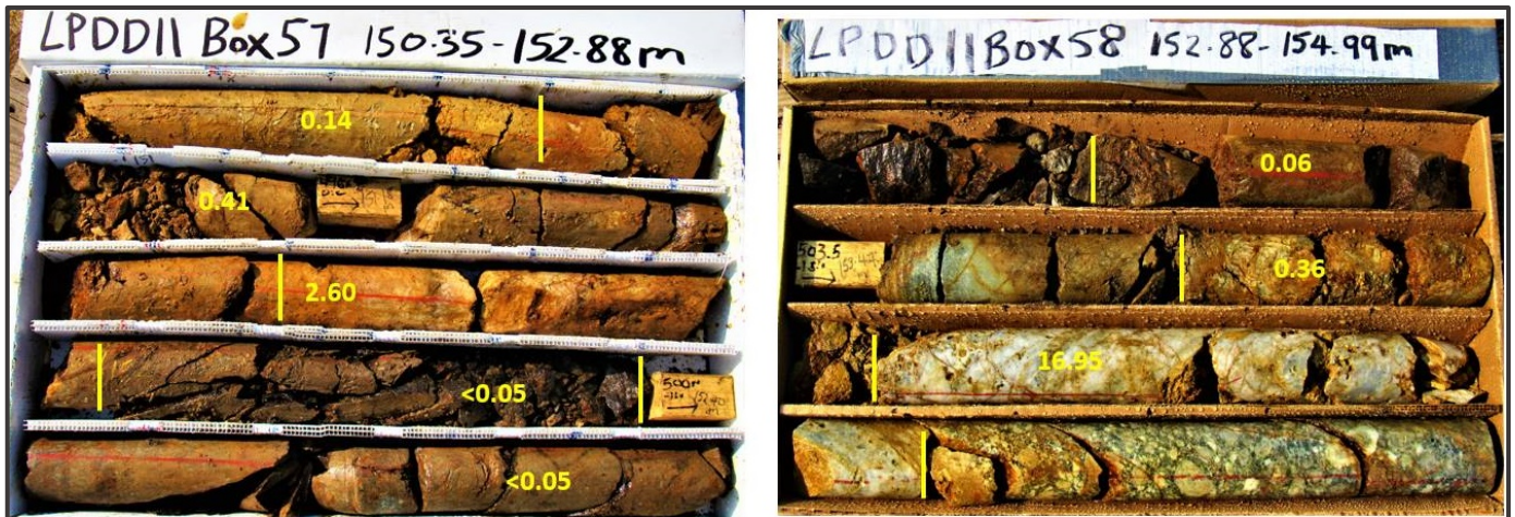
Image 2 Quartz Vein Zone – LPDD11, HQ3 Core (Core boxes hold 5ft maximum)
