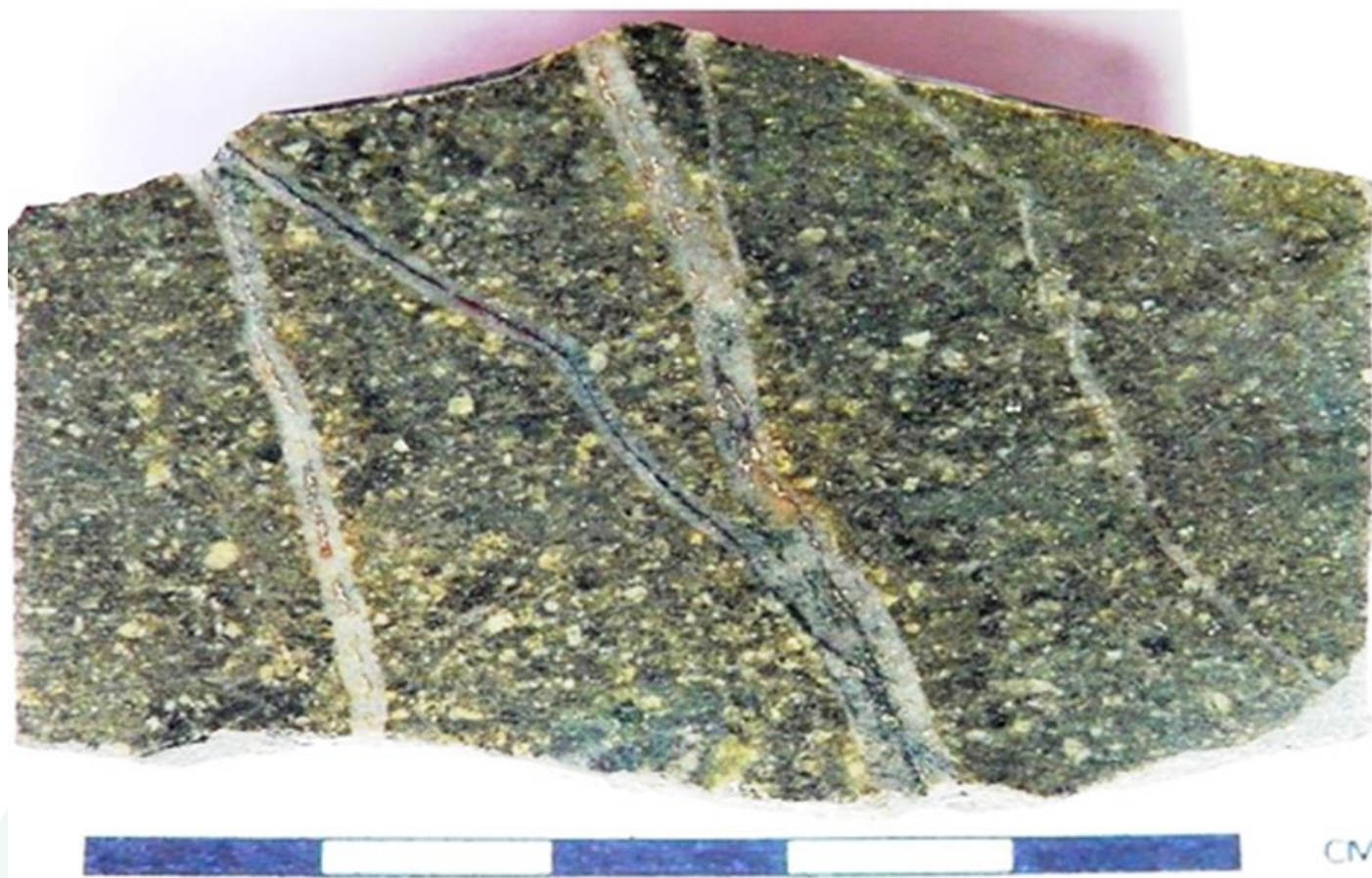
Figure 5 - Quartz-diorite porphyry, cut by banded quartz-sulphide-magnetite veins at surface
