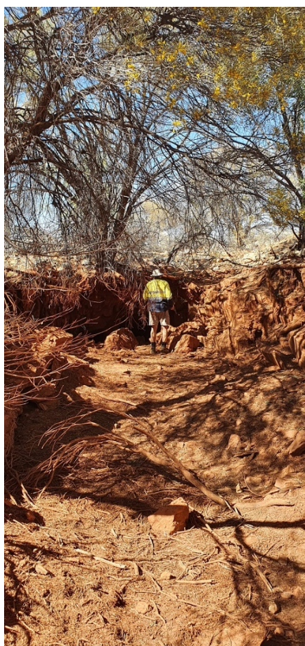
Photos 1 & 2: Examples of trenches and a shaft from Cracker Jack project (P20/2289), indicating the targeting of epigenetic gold mineralisation over a ~300m zone.
