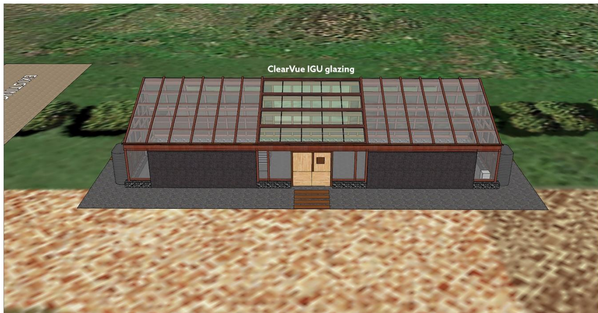
Architects rendering showing anticipated deployment of ClearVue PV IGUs into central section of sustainable greenhouse.
