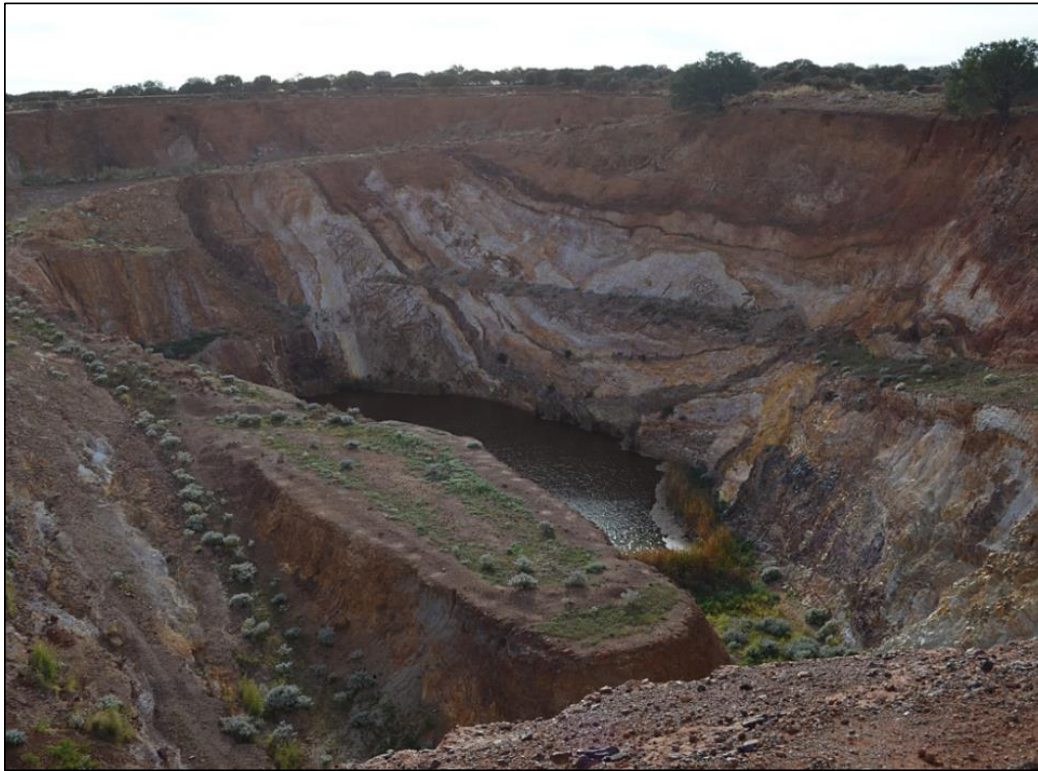
Figure 11 View of Cable mine showing narrow BIF units in the eastern pit wall.
