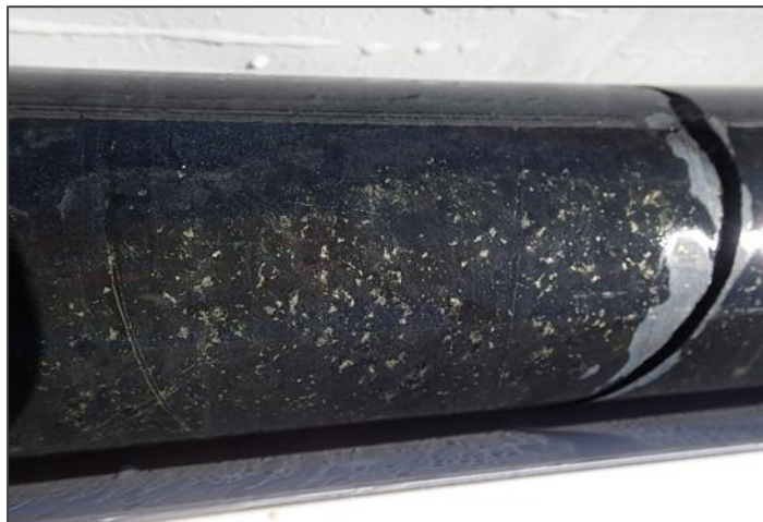
Drill core from PRDD002 with visible base metal sulphides
