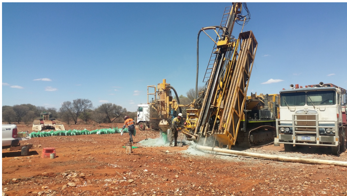
Photo 1: Larger RC rig commenced drilling of deeper hole to test depth extension
