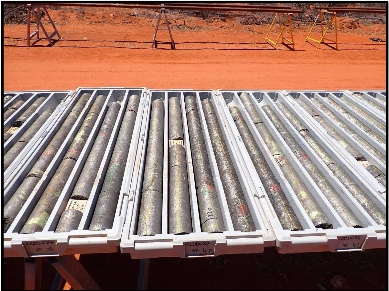
Photo 2 - Massive Ni-Cu Sulphide from the 31.1m intercept in RKDD034 to be sampled for Metallurgical test work from 220m, HQ
