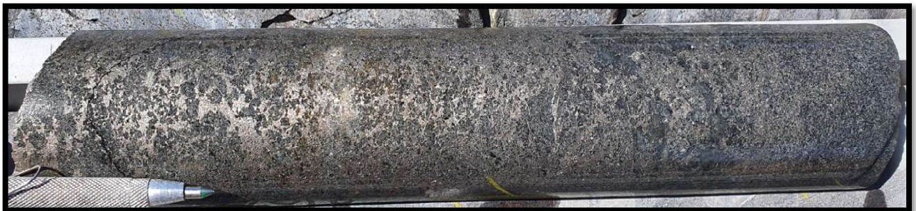
Net-texture and Heavy Disseminated Ni-Cu Sulphide from RKDD033 from 394m, NQ2
