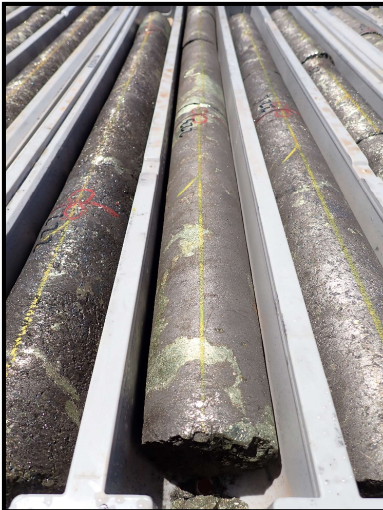
Photo 1 - Massive Ni-Cu Sulphide from RKDD034 from 223m, NQ2
