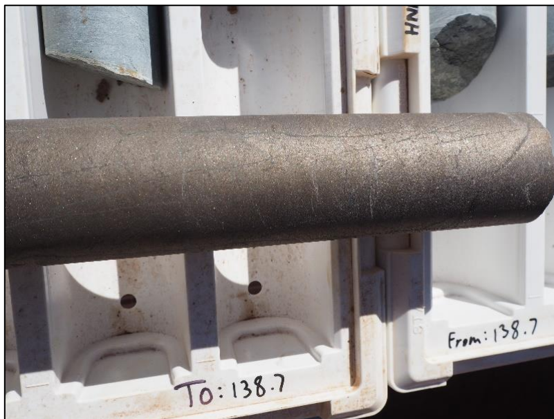
Photo 3 – Close up of nickeliferous massive sulphides (Po-Pn-Cpy) in drill core in HNDD003: assays pending
