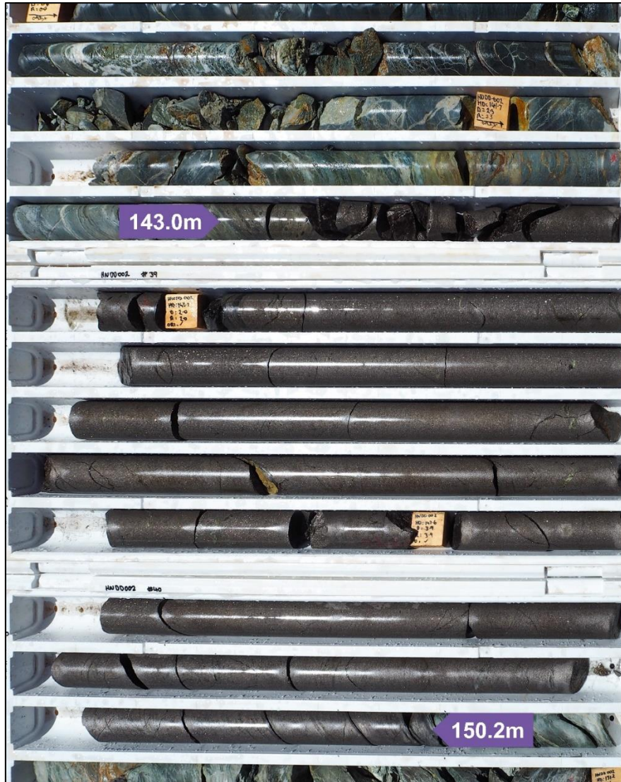
Photo 2 – HNDD002 Trays 38-40 (139.4m-151.2m): Massive nickel sulphide (Po-Pn-Cpy) mineralisation from 143.0 – 150.2m down-hole: assays pending
