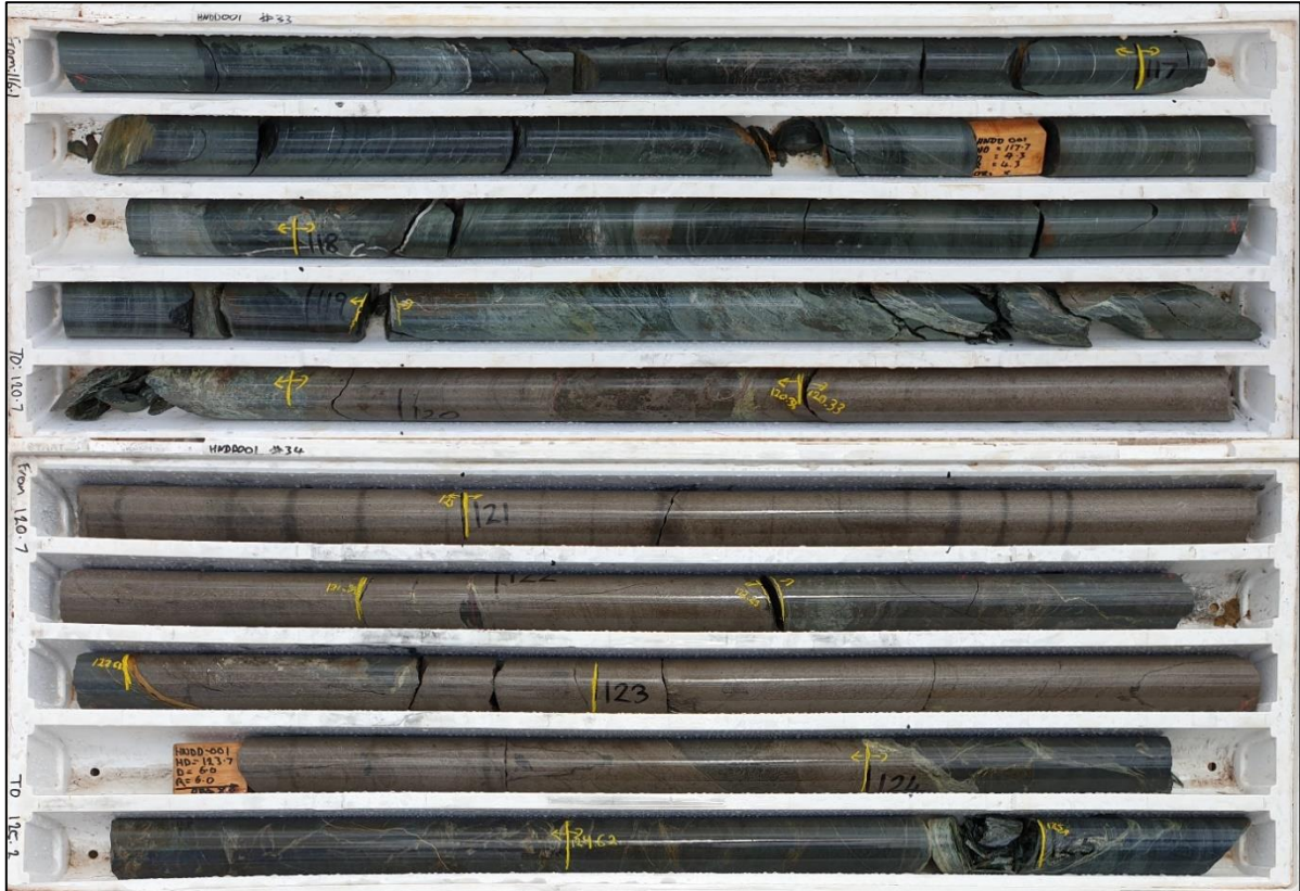
Photo 1 – HNDD001: semi-massive to massive nickel sulphide (Po-Pn-Cpy) mineralisation: 4.09m @ 2.40% Ni, 0.61% Cu, 0.55 g/t Pd & 0.22 g/t Pt from 119.91m
