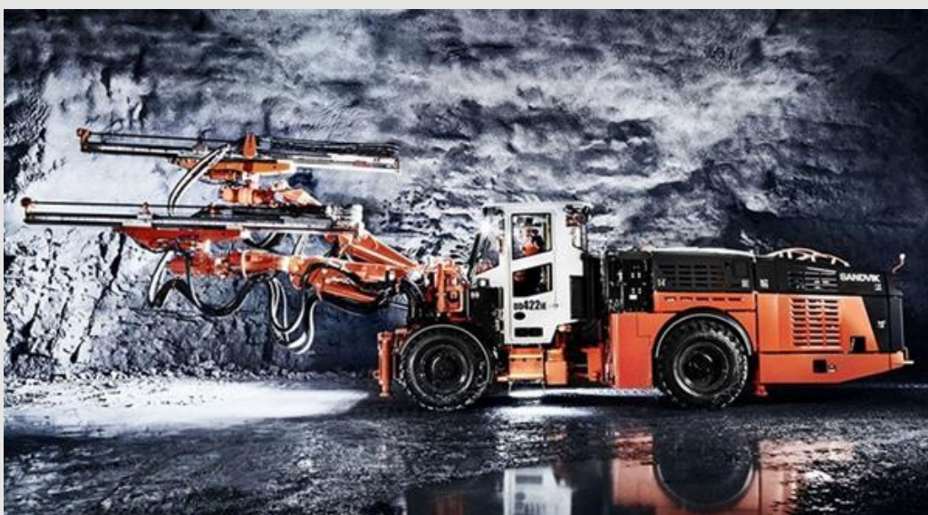
Figure 8.3 Underground development drilling Twin boom development jumbo
