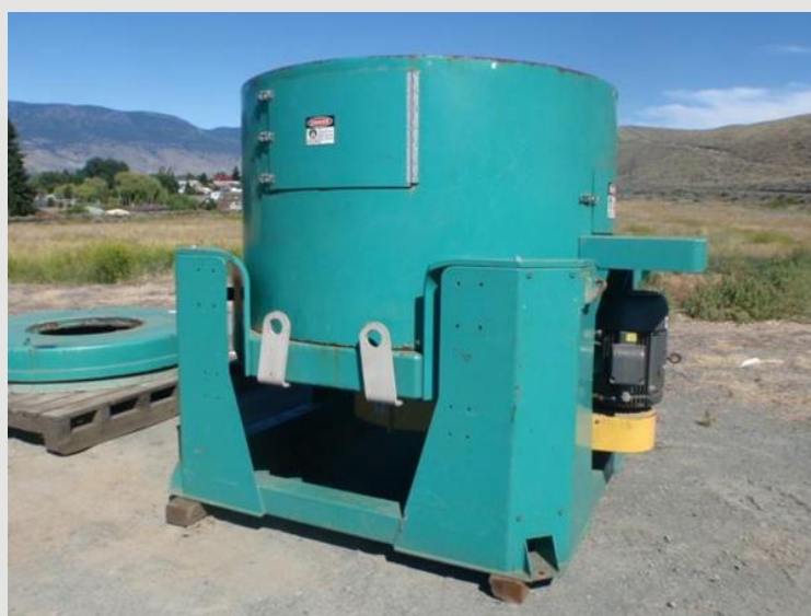
Knelson 48 CVD Hi-G centrifugal concentrator
