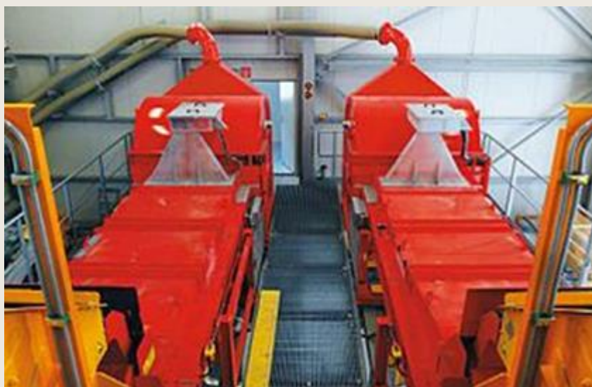
Figure 9.2 TOMRA X-Ray sorting equipment Twin XRT 1200 sorting units
