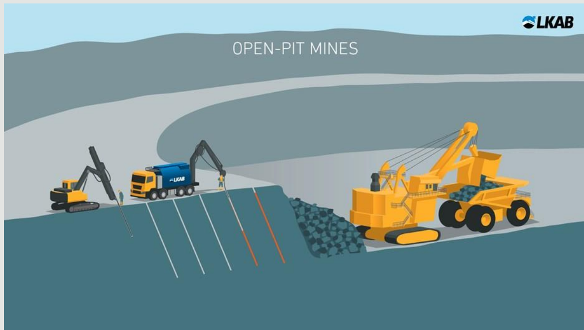
Figure 8.2 Waste drilling with face shovels and trucks
