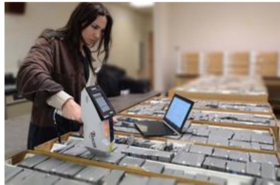
Use of a handheld X-Ray fluorescence analyser
