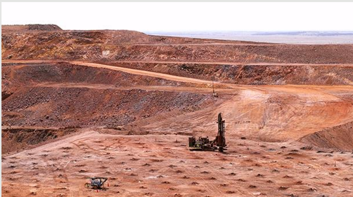
Figure 8.1 Waste drill pattern for large scale blasts
