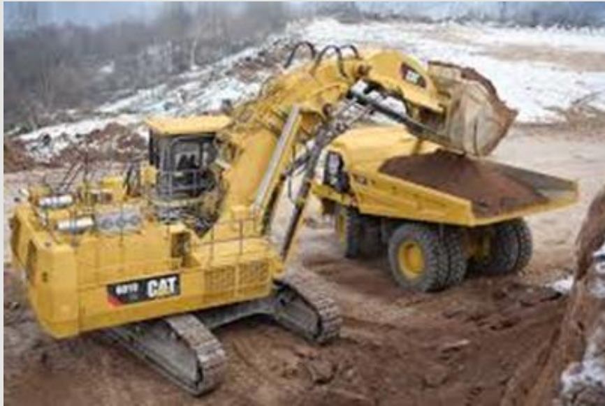
Figure 6.8 Face shovel loading waste into dump trucks on 12m benches
