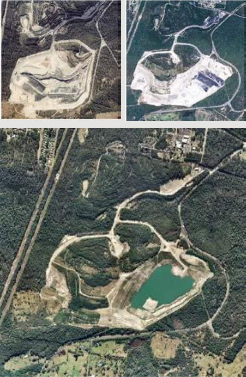
Figure 6.9 Stages of open pit reclamation from closure, recontouring and revegetation
