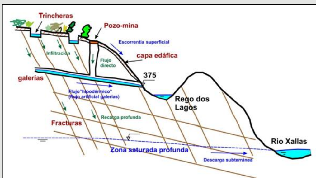
Figure 5.4 Vertical section outline of the model The model shows that the hydrodynamic system responds fast to rainfall variations (low transit time towards the adits).
