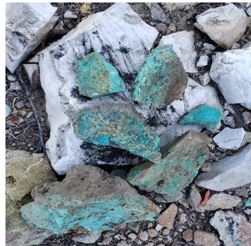
Sample DCM009 - 0.52 g/t Au, 16.05% Cu
