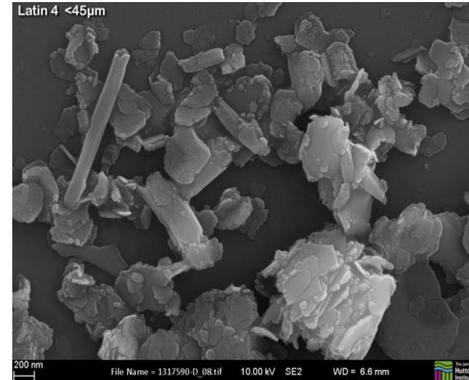
F SEMs of <45 micron fractions showing halloysite tubes and kaolinite plates from location 4
