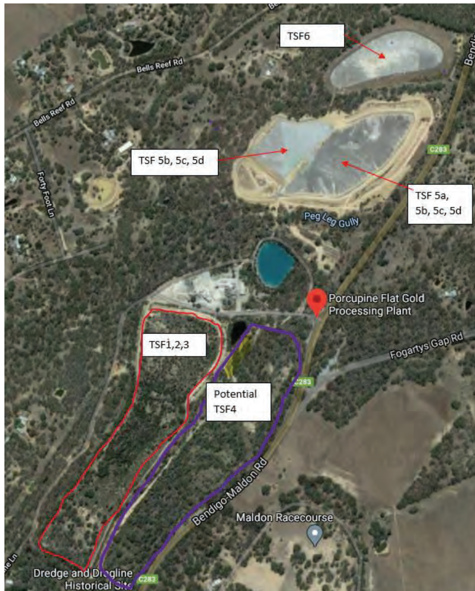
Figure 3-9 Tailings Dam Layout
