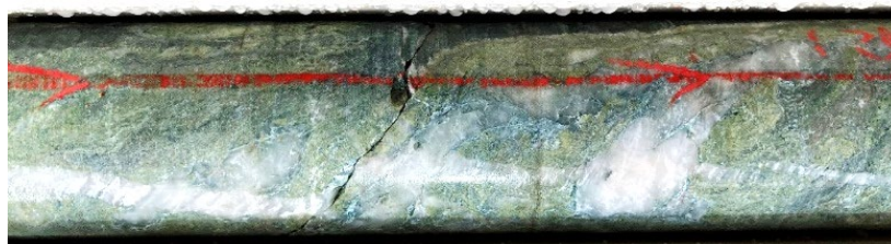
Figure 2: Quartz/carbonate/epidote/?actinolite vein (H8DD023, 374.5m, NQ core)
