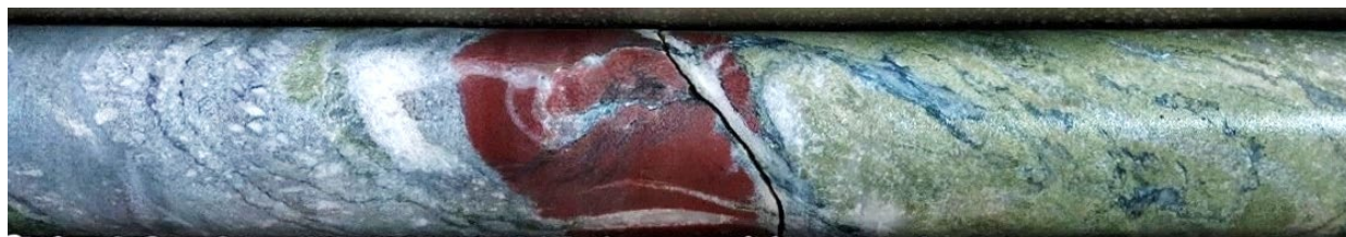
Figure 3: Quartz/carbonate/epidote/hematite vein (H8DD023, 395.4m, NQ core)
