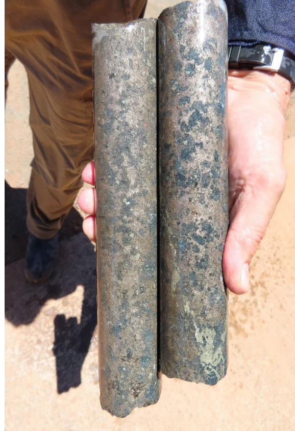
Figure 2: ANDD0004 drill core Matrix Ni-Cu sulphides @ 352.9m - 353.6m 0.7m @ 2.64% Ni & 0.27% Cu
