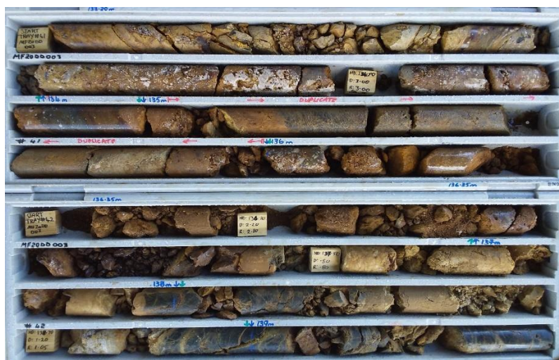
Photo 4. Section of ore zone in MF20DD003: 5 metres @ 11.24g/t Au from 133-138m incl. 3m @ 18.59g/t Au.
