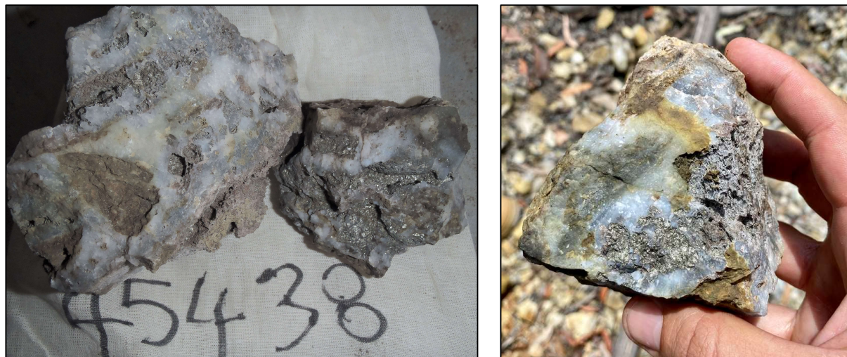
Figure 1: (left) Historic rock chip sample 45438 returned 5.62 g/t Au (right). New field mapping confirms presence of quartz – arsenopyrite breccia at Bonneville.
