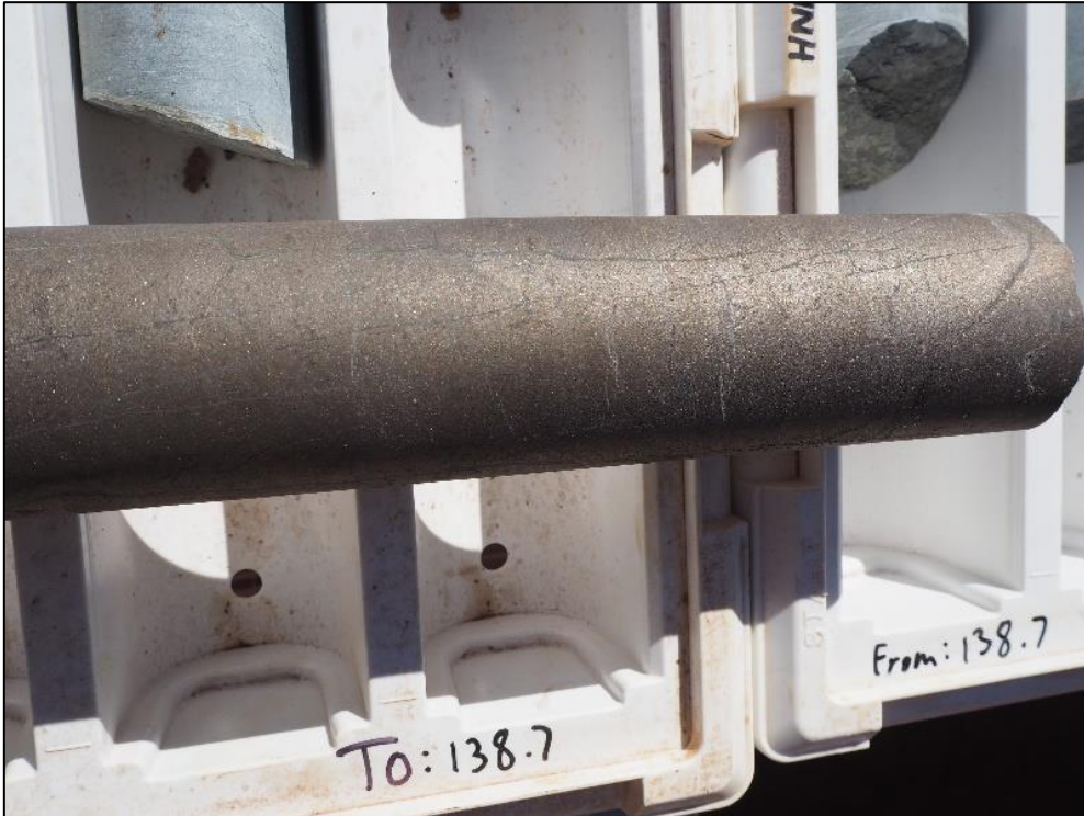
Photo 2 – Close up of nickeliferous massive sulphides in drill core in HNDD003: 2.41% Ni, 0.47% Cu and 0.46g/t Pd
