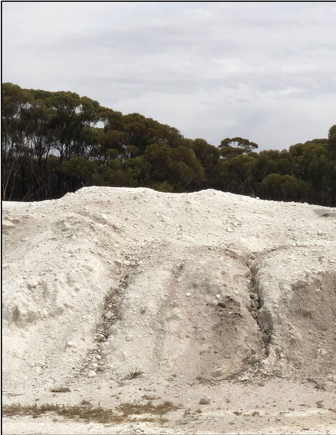
Figure 4 – Photo showing bright white kaolinitic clays and kaolinized granite in dam walls at sample Location WD02-1
