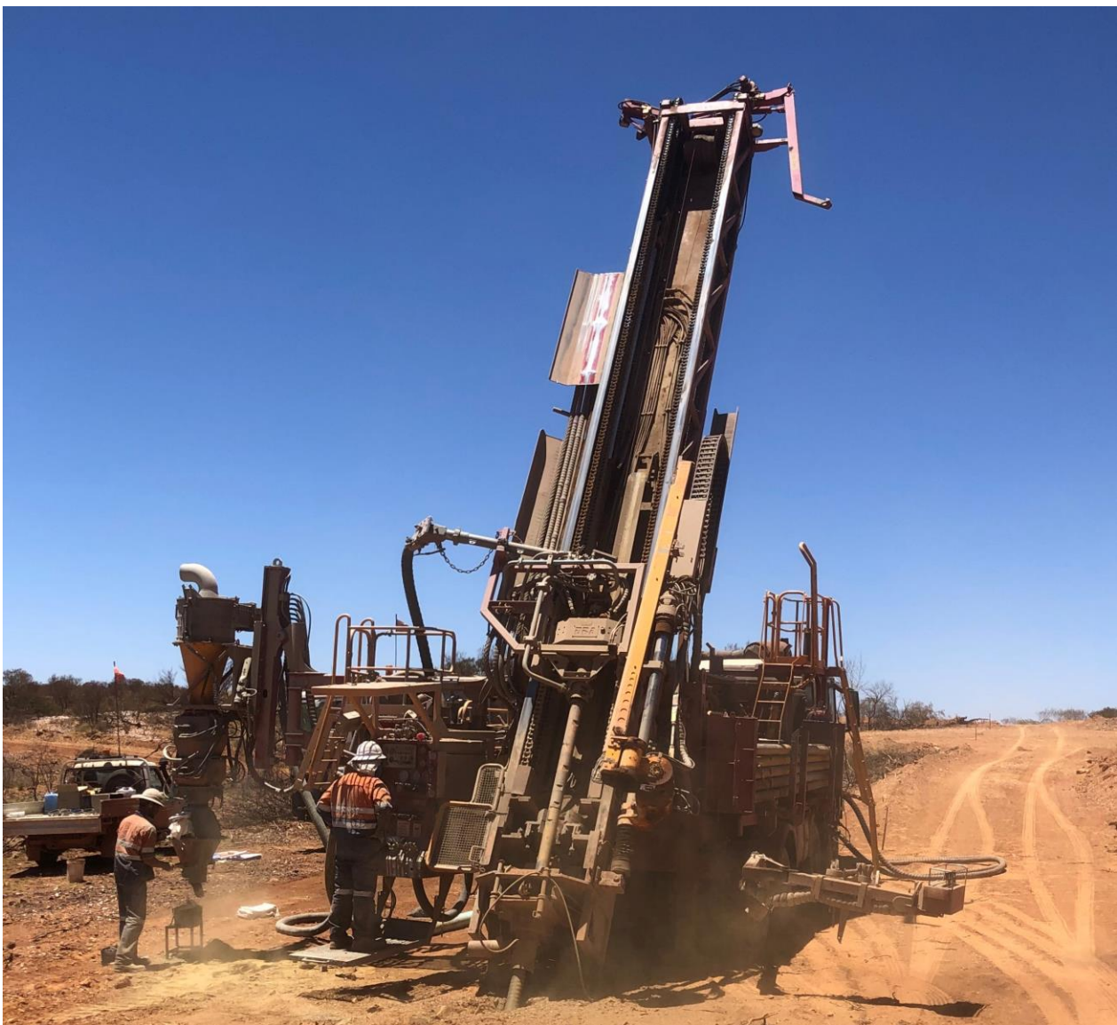
Figure 3: The RC Rig collaring at Saltwater mining area in preparation for drilling, targeting old worked areas from the 1980s.
