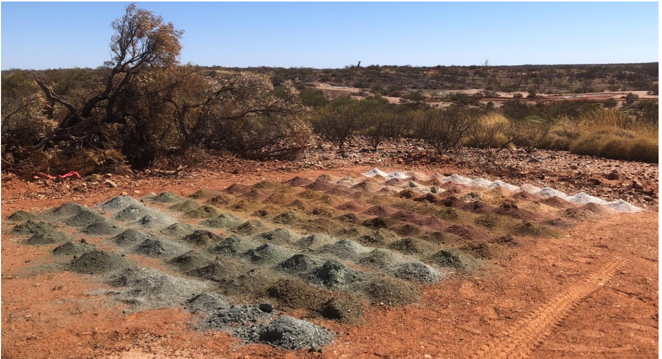
Figure 4: Sample piles showing the 12m of younger chert cover (right) and pale alteration zones
