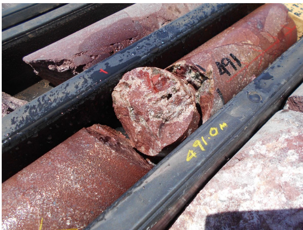
Above and Below: DD20EB0002 encountered haematitic fault breccia within the Pandurra Fm. Copper sulphides were logged in vugs, with elevated copper grades confirmed by portable XRF, confirming the fault as having carried copper and iron bearing fluids.
