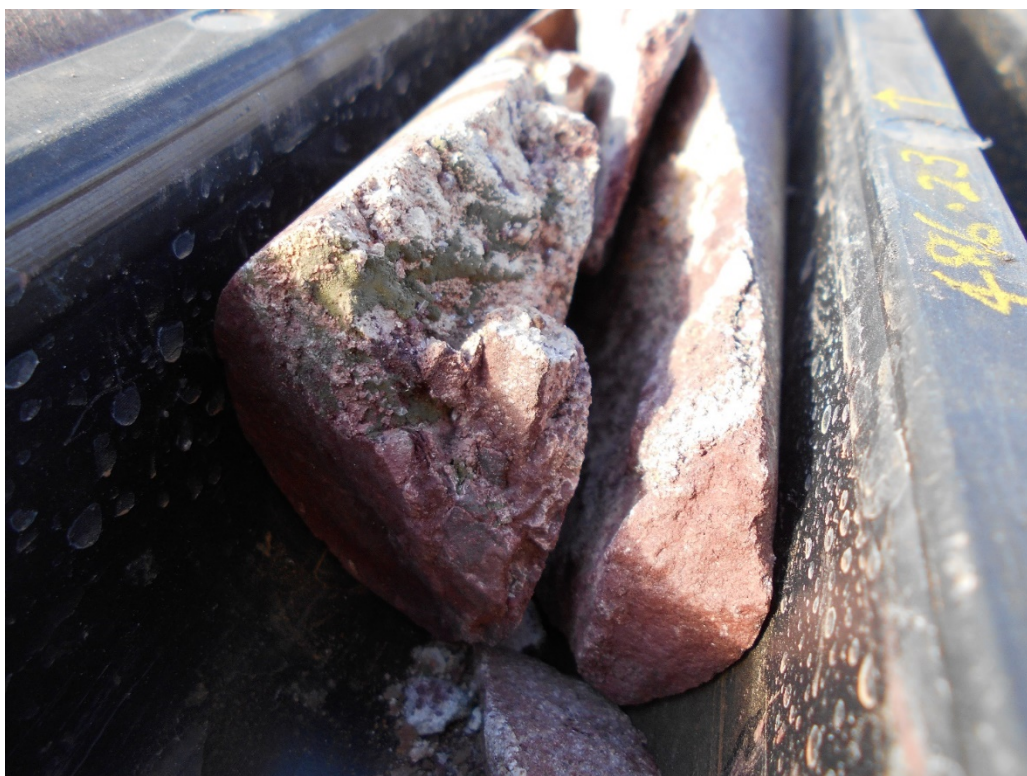
Above and Below: Copper sulphides are irregularly distributed through the breccia, and are most prominent in vugs, on fracture surfaces and associated with quartz veining.
