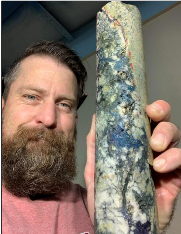
Figure 2 Eagle Mountain's Brian Paull, Principal Geologist in Arizona with a section of bornite -rich core from the mineralised breccia in hole WT-20-06 (From 210 to 212.95m down hole). The core is part of a high-grade interval assaying 6.67% Cu, 63.5g/t Ag and 0.87g/t Au over 2.95m
