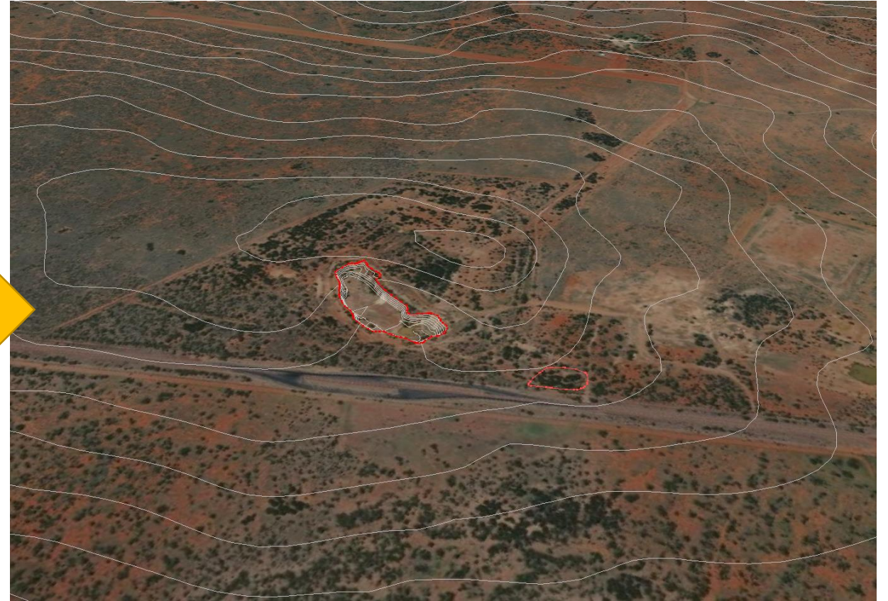
6. Draped high res satellite imagery yielding working 3D topography with accuracy sub- 1m in x and y, and sub- 2m in z, to validate historic data and facilitate forward programme design
