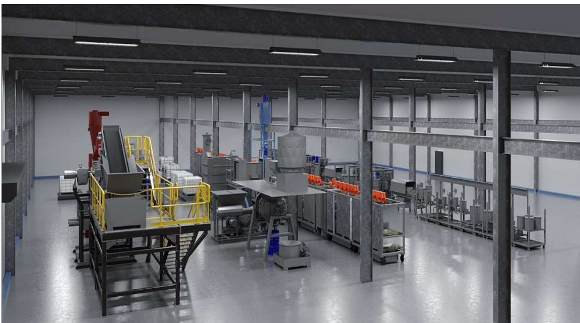
Figure 1 - Render of demonstration plant in Hilchenbach showing battery shredding (left, foreground) and hydrometallurgical refining circuits (right, background)
