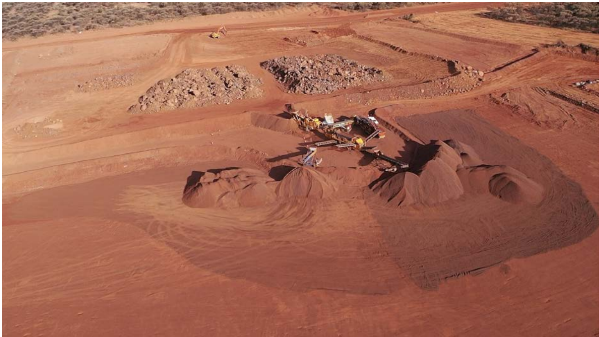
Figure 1: High-grade ore crushed and stockpiled on ROM pad awaiting transport.
