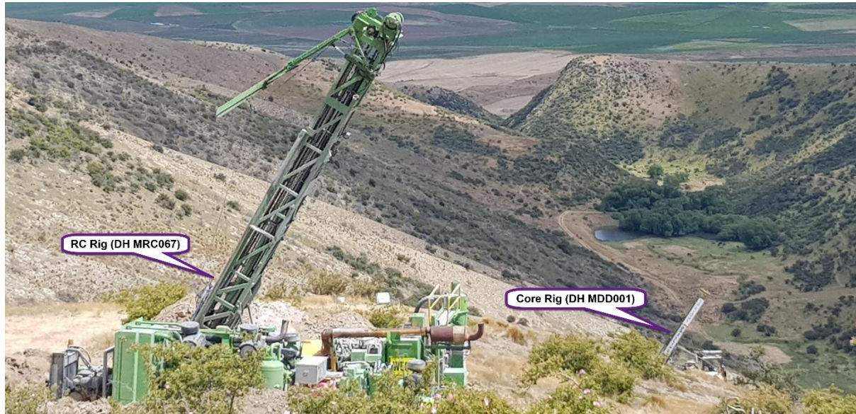
Figure 4 Come-in-Time (CIT) drilling (view NW)– RC and DD rigs drilling in tandem
