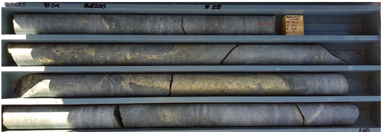
Image 6 | NWD2003 drill core 95.5m to 99.0m downhole showing chalcopyrite and pyrrhotite mineralisation
