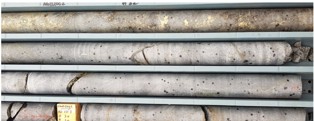
Image 3 | NWD2002 drill core 108.0m to 108.8m downhole showing chalcopyrite and pyrrhotite mineralisation
