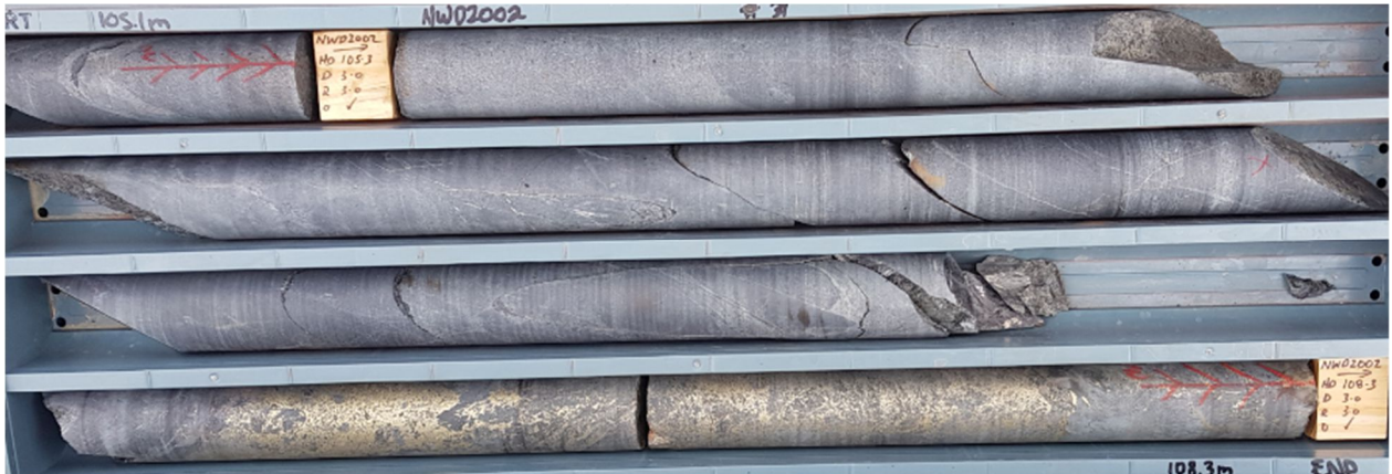
Image 4 | NWD2002 (drill core 107.5m to 108.0m downhole showing chalcopyrite and pyrrhotite mineralisation)
