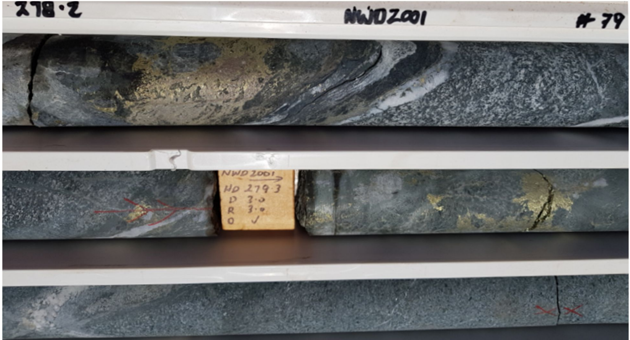
Image 2 | NWD2001 drill core 278.2m to 279.3m downhole showing chalcopyrite and pyrrhotite mineralisation
