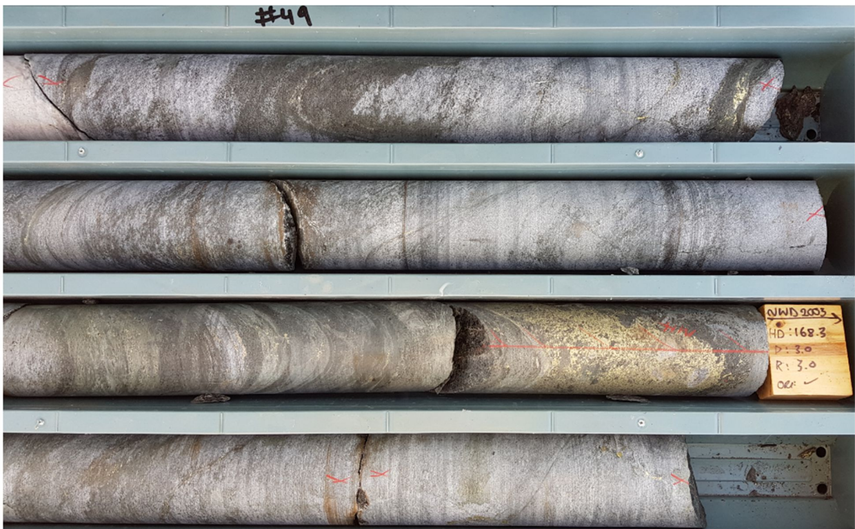
Image 5 | NWD2003 drill core 168.1m to 168.3m downhole showing chalcopyrite and pyrrhotite mineralisation
