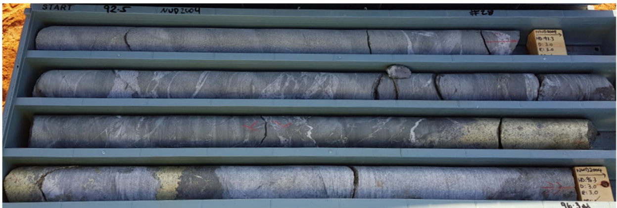
Image 7 | NWD2004 drill core 92.5m to 96.3m downhole showing chalcopyrite copper sulphide mineralisation
