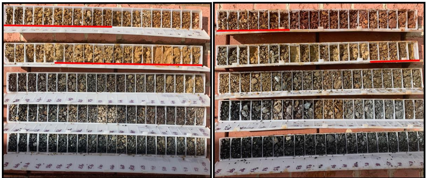
Photo 1: RC Chips from BJRC003 (Left) and BJRC004 (Right), showing zones of anomalous copper (Red lines) in strongly weathered bedrock in each hole.
