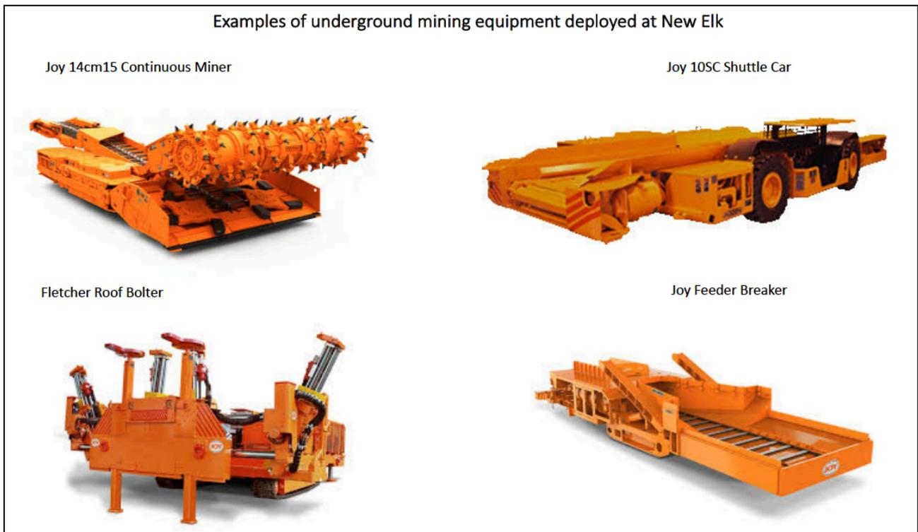
Image: examples of the main items of equipment in a room and pillar operation
