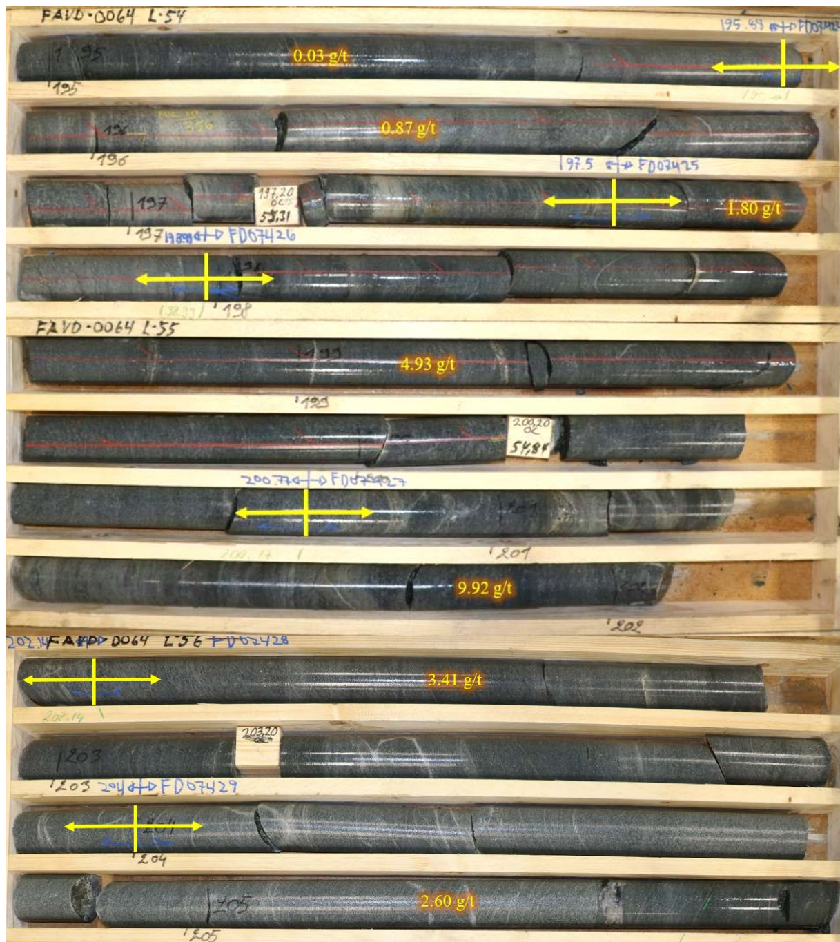
Figure 6. Core photographs of higher grade mineralisation in hole FAVD0064 showing 2m composite gold assay results.
